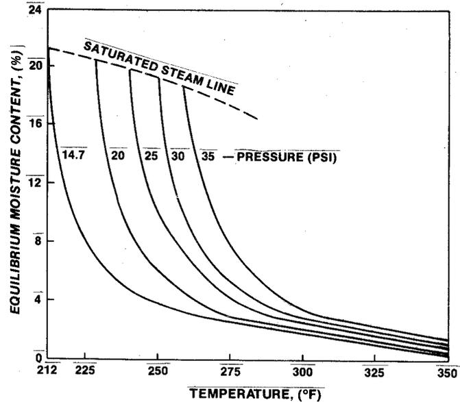
Figure 2. Equilibrium moisture content of wood versus temperature at various pressures. Curves are derived from data by Keylwerth (5) at atmospheric pressure (14.7 psi) and by Engelhardt (2) above atmospheric pressure.
