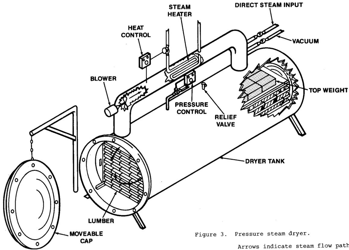
Figure 3. Pressure steam dryer.
