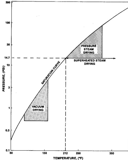
Figure 1. Pressure-temperature diagram for steam showing saturation curve and operating regions for vacuum, superheated steam, and pressure steam drying.
