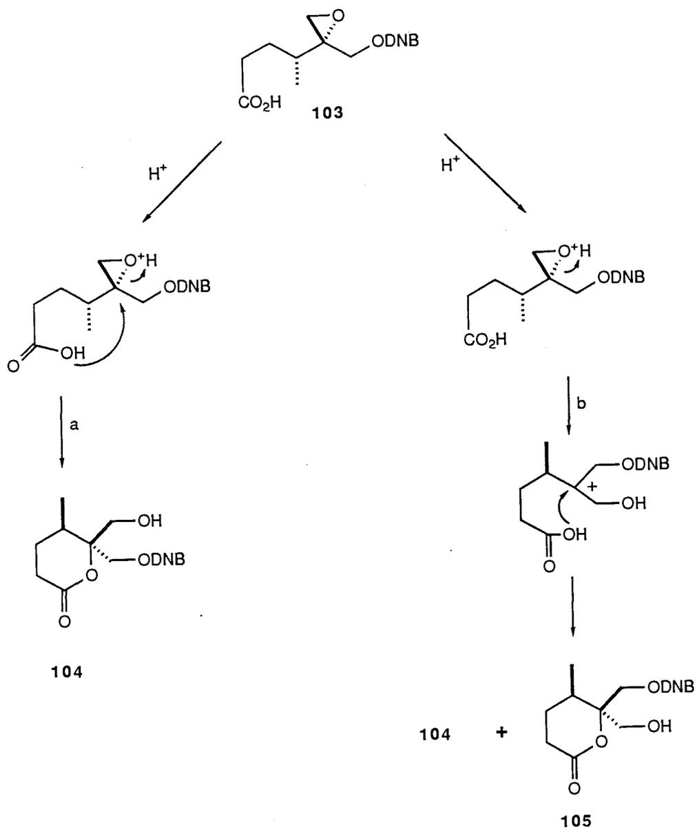
Figure 5. Proposed mechanism for the acid catalyzed epoxide opening.
