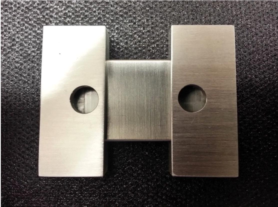
Figure 3.20: SCO2 Circular Channel Design: Photograph of assembled device prior to welding of the three parts and inlet and outlet tubes.
