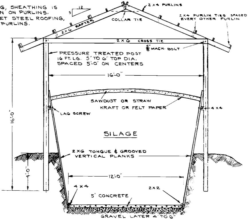
CROSS SECTION OF TRENCH SILO WITH CREOSOTED PLANK-LINED CONSTRUCTION
