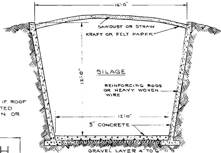
CROSS SECTION OF TRENCH SILO WITH REINFORCED CONCRETE WALLS
