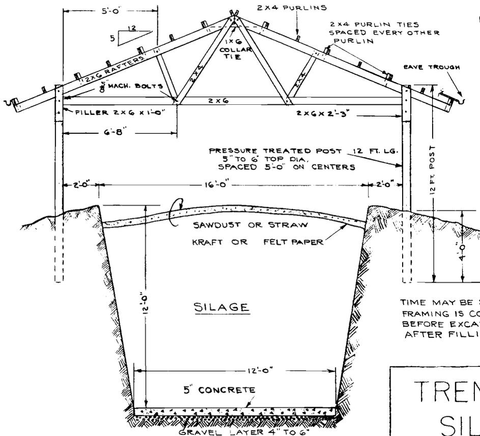
FOR ASPHALT ROOFING, SHEATHING IS APPLIED UP AND DOWN ON PURLINS.
