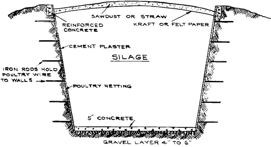
CROSS SECTION OF TRENCH SILO WITH REINFORCED CONCRETE CURB AND PLASTER LINED
