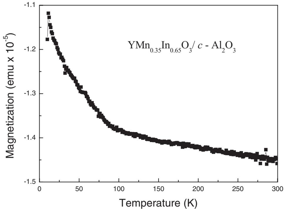
FIG. 2. Field cool magnetic moment as a function of temperature with a magnetic field of 1 kOe.
