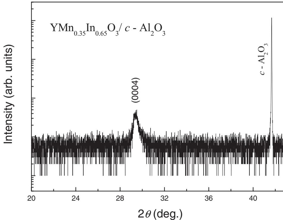
FIG. 1. X-ray diffraction pattern shows the *c*-oriented growth of  $\text{YMn}_{0.35}\text{In}_{0.65}\text{O}_3$  thin film.
