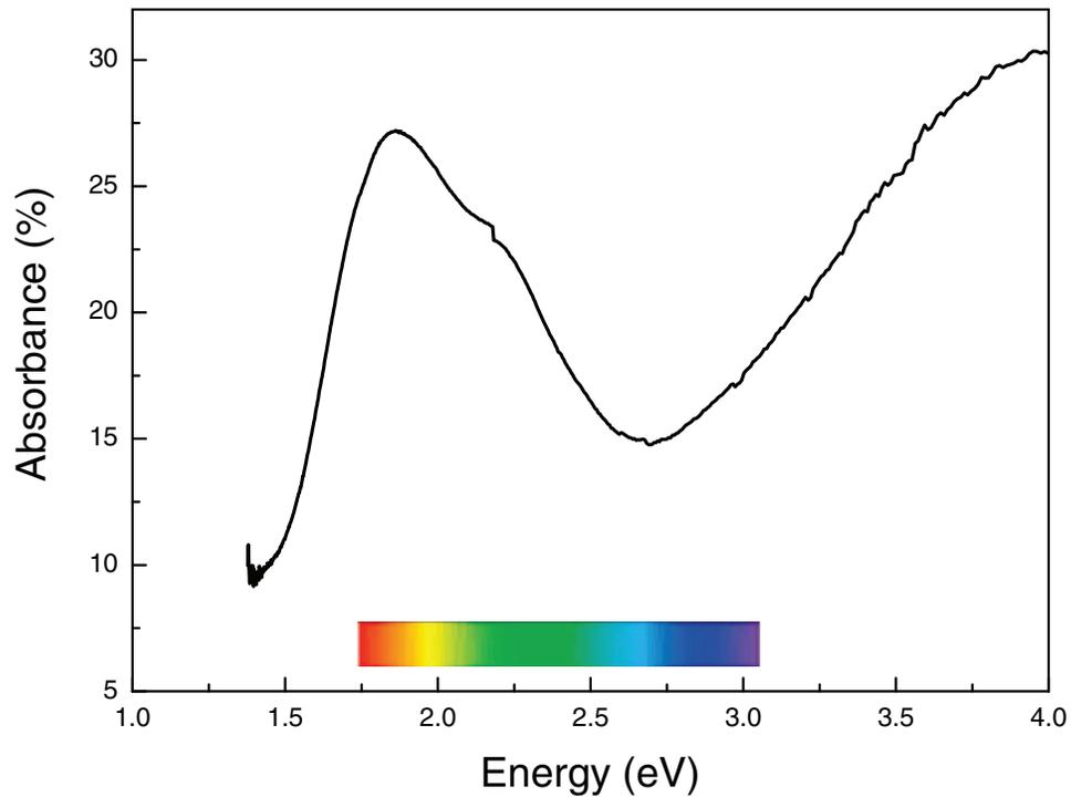
FIG. 3. Absorbance spectrum of  $\text{YMn}_{0.35}\text{In}_{0.65}\text{O}_3$  film in the visible region.
