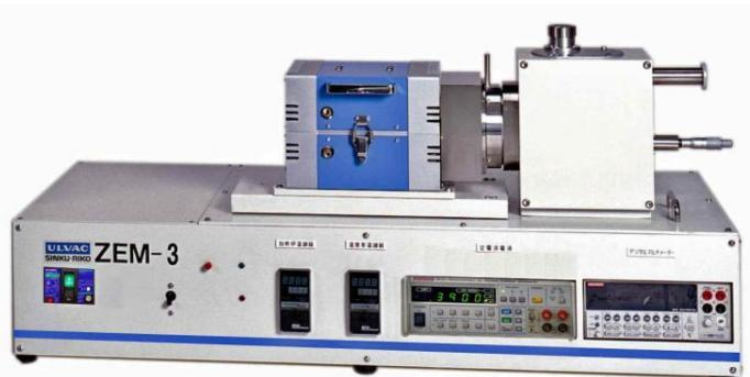
ZEM used to measure electrical resistivity and Seebeck coefficient from 200-500 °C
