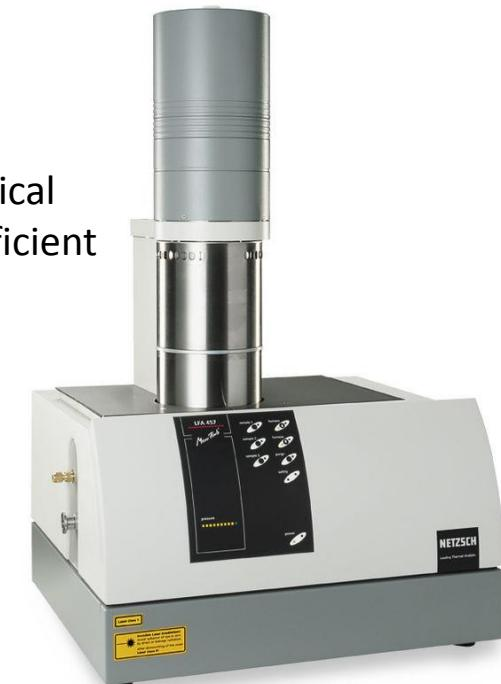
NETZSCH LaserFlash used to measure thermal diffusivity from 50-500 °C
