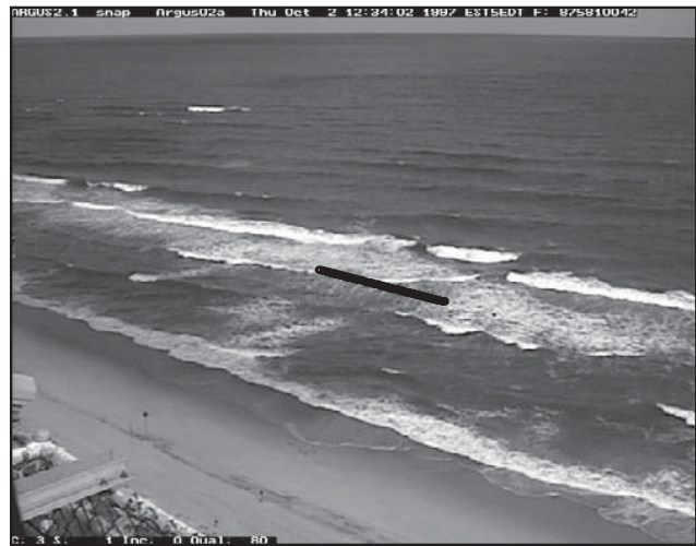
Figure 1. Snapshot of the surf zone at Duck, North Carolina, on 2 October 1997. The line indicates the location of an alongshore pixel array where video record (Figure 2) was taken.
