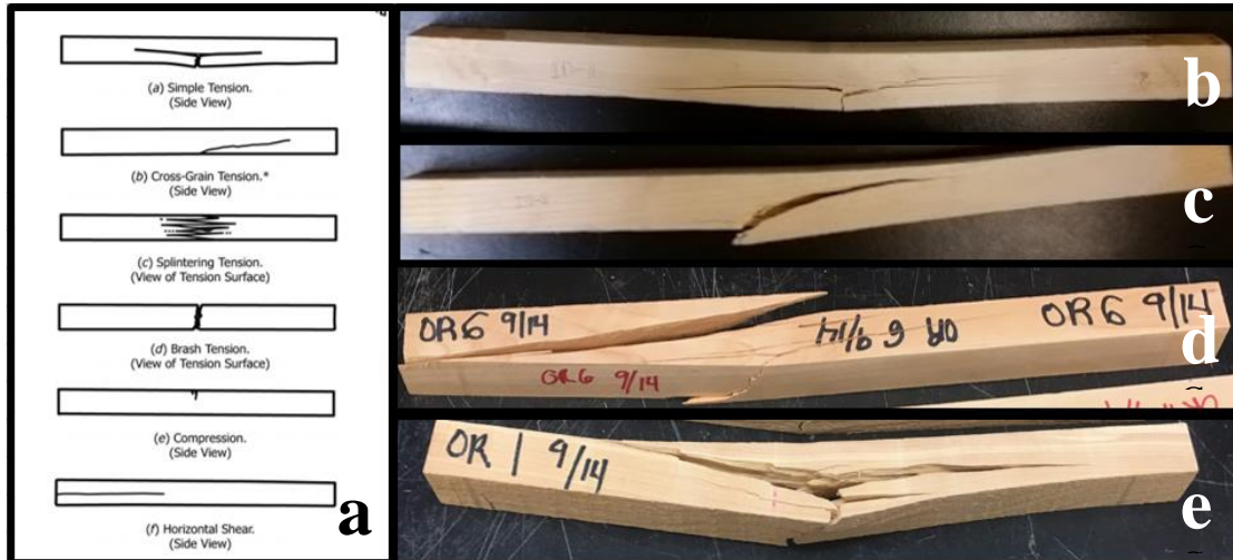
Figure 19: Three-point bending failures showing (a) Common failure types noted in ASTM Standard D143 (b) Simple tension failure (most common failure) (c) Cross-Grain Tension (d) Horizontal Shear (e) Catastrophic simple tension failure
