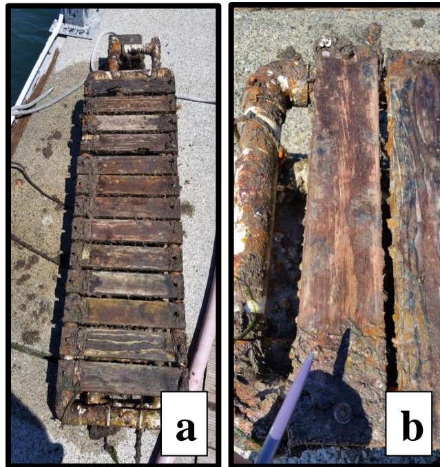
Figure 8: Example of a (a) Marine borer test racks. (b) and a western juniper sample attacked by marine borers (6-month exposure).
