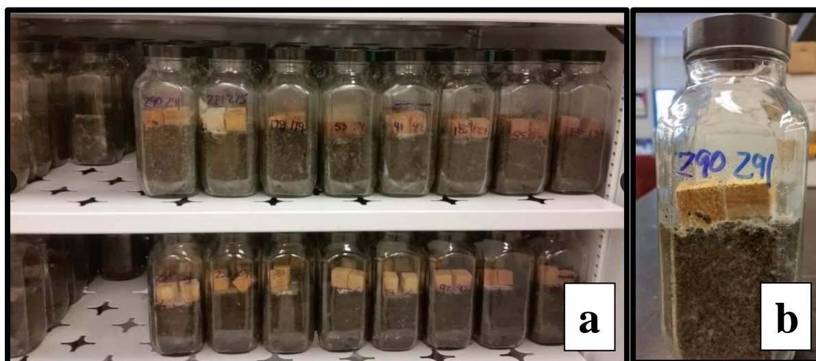
Figure 9: Soil Block Test. (a) Soil block jars in incubator. (b) Soil block jar after 16-week incubation period
