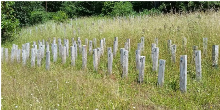
Figure 10: Ground Contact Samples at the Peavy test site
