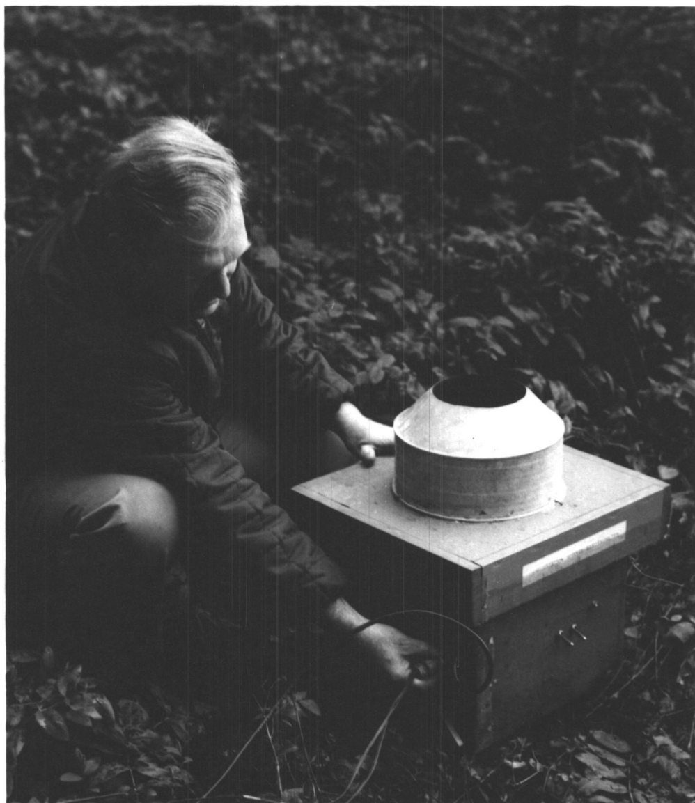
Fig. 4 PRECIPITATION CHARGE ELECTRO- METER IN THE FIELD
