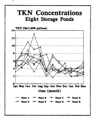
The summer months contain a higher concentration of TKN than the winter months. This may be due to the increased biologic activity of the pond, as bacteria are breaking down or digesting organic material that has settled near the bottom of the pond. As this organic layer is digested, some organic matter rises into the liquid, thus increasing the concentration of the wastewater.
