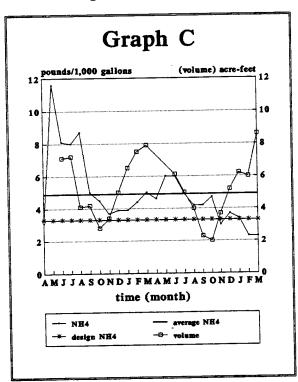
In pond B, there is an inverse relationship between pond volume and NH<sub>4</sub> concentration. Note that when the NH<sub>4</sub> concentration is relatively high, the pond volume is relatively low. This is due to dilution of additional water into the storage pond, lowering the NH<sub>4</sub> concentration.
