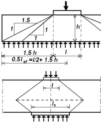
Fig. 6: Assumed dispersion of stresses for two load cases
