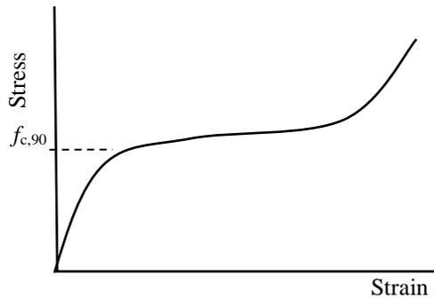
Fig. 2: Stress-strain curve perp. to grain of wood.
