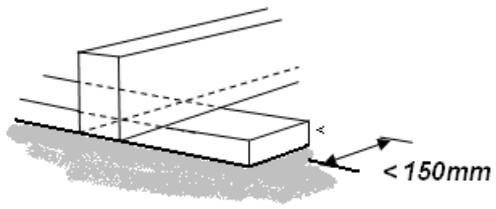
Fig. 5: Bearing on continuous support
