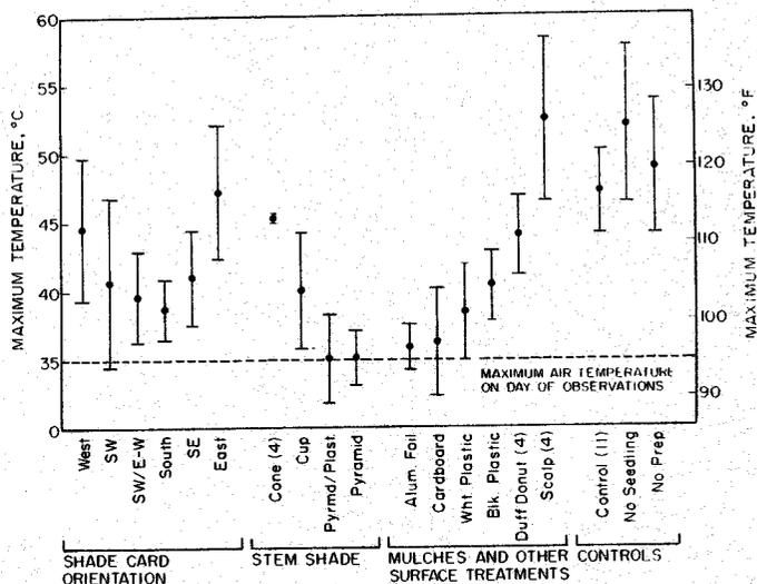
Figure 1. Maximum soil temperatures at 2 cm depth, by treatment, August 24, 1982.
