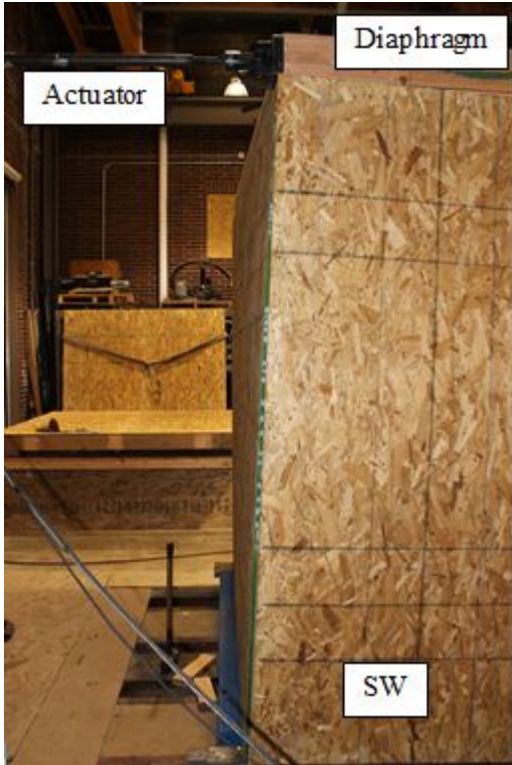
Fig. 7: FAIL2 loading setup
