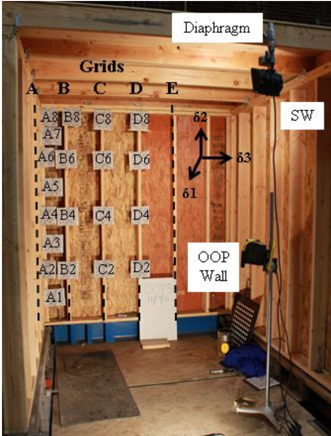
Fig. 5: Test setup 2C with grids and targets
