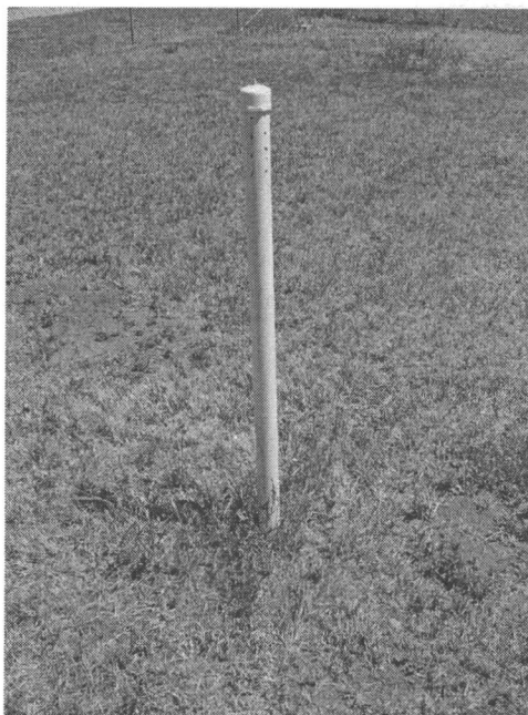
Figure C.2: Ambient only thermal probe station, approximately 1 m above ground level. Data logger is suspended within the cap portion of the station. Thermal probe station was perforated to allow free air passage.
