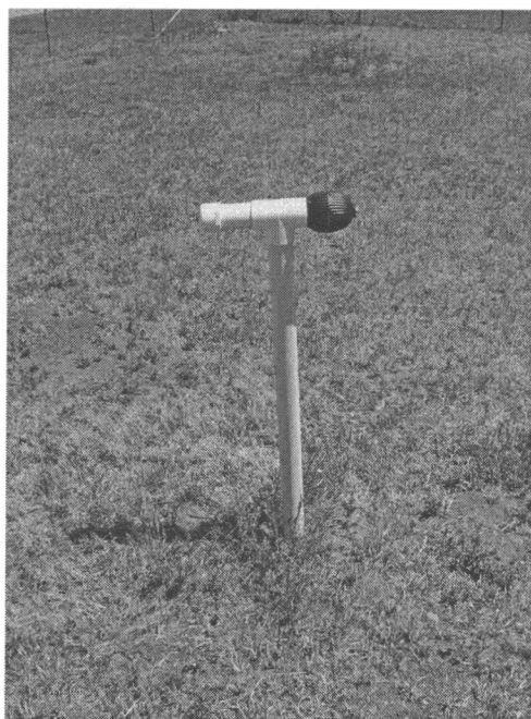
Figure C.2: Ambient only thermal probe station, approximately 1 m above ground level. Data logger is suspended within the cap portion of the station. Thermal probe station was perforated to allow free air passage.
