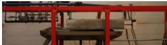
Figure 3.5-1: Trolley in the heating position, where the heater is in the center of the image and the cooling manifold is in the upper left corner of the image.
