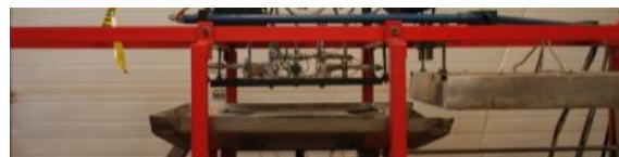
Figure 3.5-5: Trolley in cooling position, where the nozzles are over the test plate.
