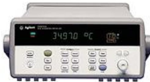
Figure 4.6-1: Picture of the Agilent data boxed used in the data collection (42).
