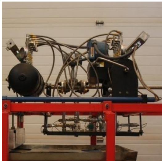
Figure 3.4-7: Picture of the gas (left) and liquid (right) distribution tanks, valves and flow meters. The tank and valves on the left distribute the gas and the tank and valves on the right distribute the liquid to the nozzles. Picture shown with two-phase nozzles installed.
