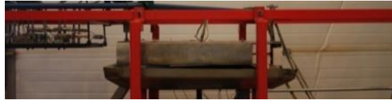
Figure 3.5-1: Trolley in the heating position, where the heater is in the center of the image and the cooling manifold is in the upper left corner of the image.
