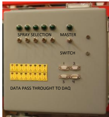
Figure 3.4-6: Figure of the fluid control and DAS wiring cabinet.
