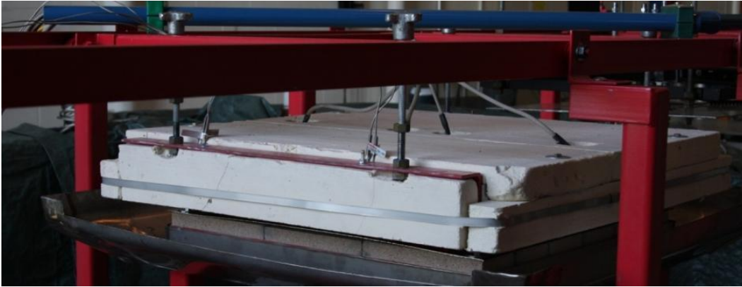
Figure 3.4-3: Picture of the heaters installed on the trolley. The heater is shown with 2" thick calcium silicate insulation.
