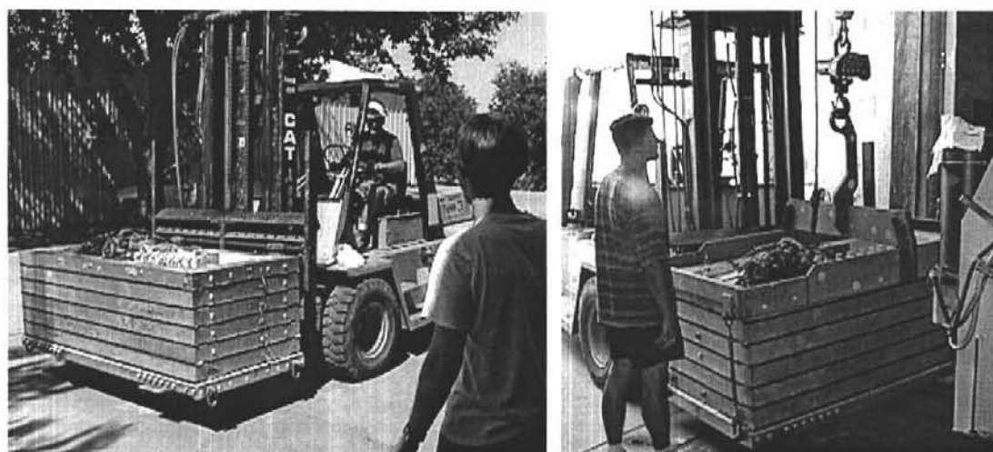
Figure 5-10: Moving the model box and placing it on the centrifuge arm
