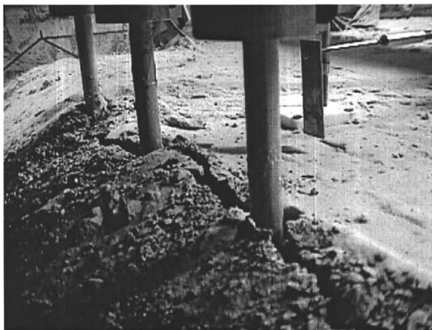
Figure 10-10: Pile gapping and deformation cracks after all earthquakes in test NJM02.
