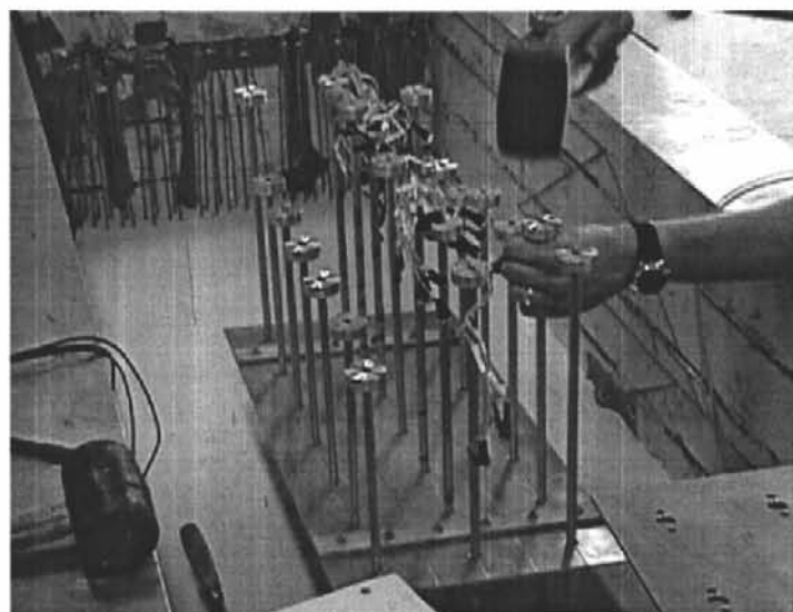
Figure 5-7: Driving the piles through the template with a rubber mallet (NJM02)
