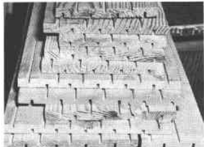
Figure 5. Lumber grooved on alternate sides before panel assembly.
