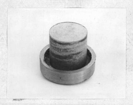
Figure 2. Compact of Zirconium-Hydride Powder and Magnesium Shavings in Iron Crucible.
