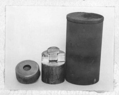
Figure 8. Cutaway View of Magnesium-Zirconium Diffusion Specimen with Carbon Crucible.
