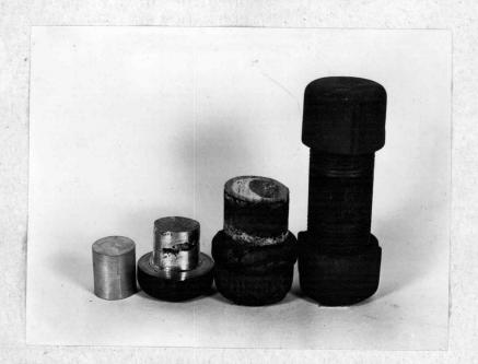
Figure 3. Steel Bomb, used for making Magnesium-Zirconium Alloy, with Finished Ingot of Magnesium-Zirconium.
