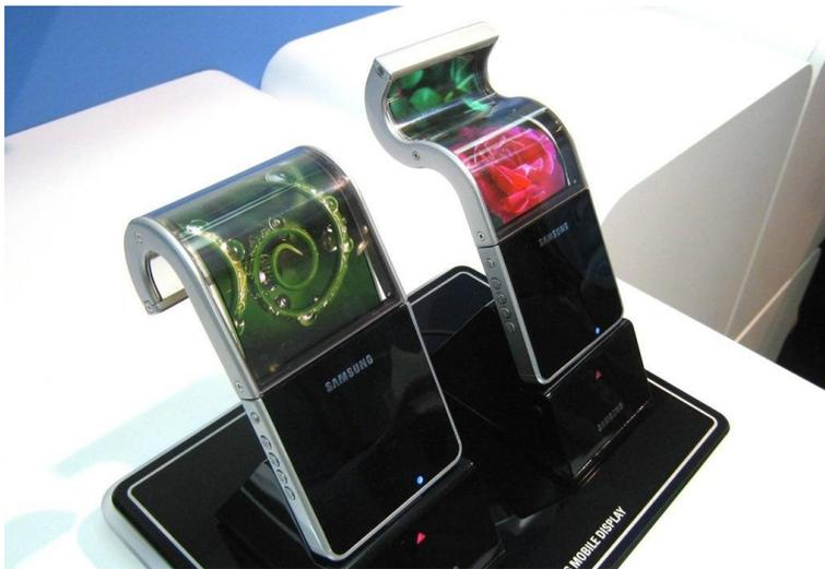
Figure 1.1: Patented concept and Prototype for Samsung’s new flexible AMOLED OLED display. Flexible displays are created by “printing” organic semiconductors onto a substrate between cathode and anode layers [1].
