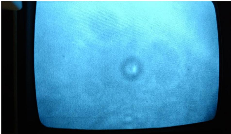
Figure 2.9: Coated micro-sphere trapped in optical tweezers with trapping laser filtered out with IR filter. Feed from CCD camera displayed on viewing screen.
