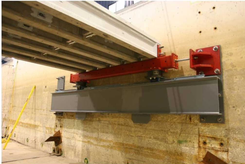
Figure 3-6. Photo of rigid test setup installed in Large Wave Flume. In this photo, the horizontal load cell between the bent cap and the end anchorage block has been temporarily replaced by a 1" threaded steel rod.
