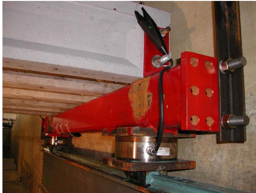
Figure 3-9. Photo of installed vertical load cell, LC5. LC4 can be seen in the background.
