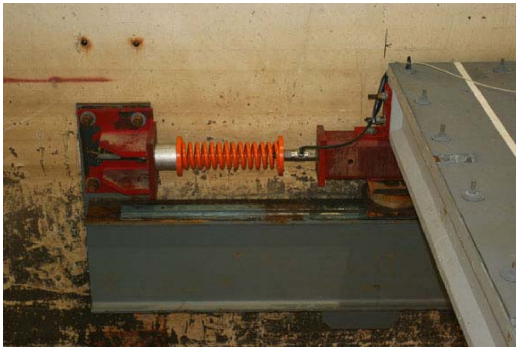
Figure 3-7. Photos of stiff (top photo) and soft (bottom photo) springs installed with horizontal load cell, LC2.
