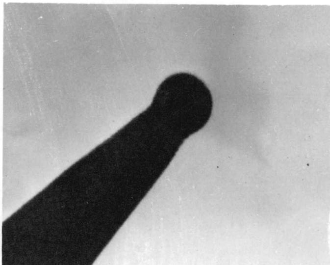
Fig. 43 Emitter point after use. Magnification 1500x.
