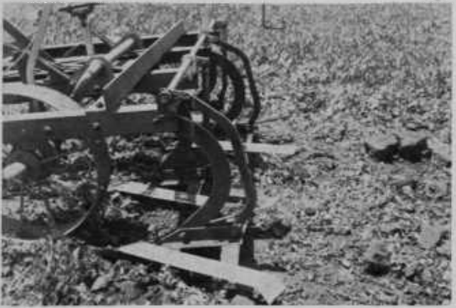
SWEEP PLOW for making initial tillage.
