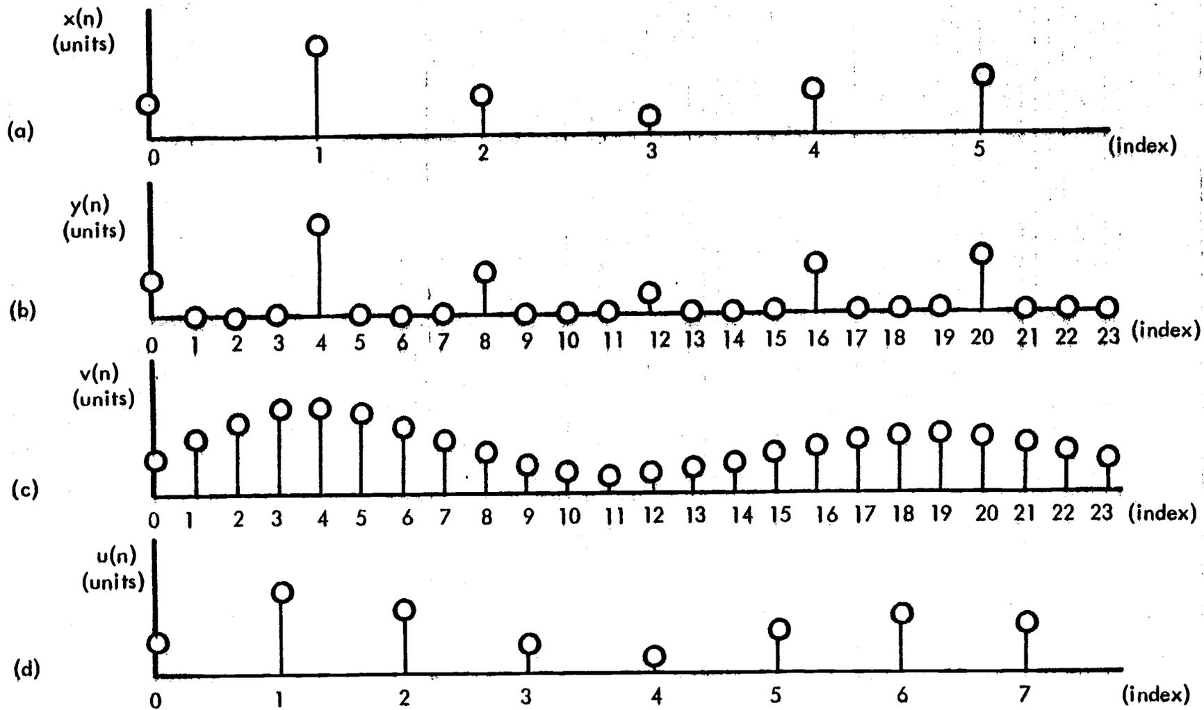
Fig. 8 (a) Original sequence. (b)  $x(n)$  interpolated by 4. (c) typical response when  $y(n)$  is low pass filtered. (d)  $v(n)$  decimated by 3.
