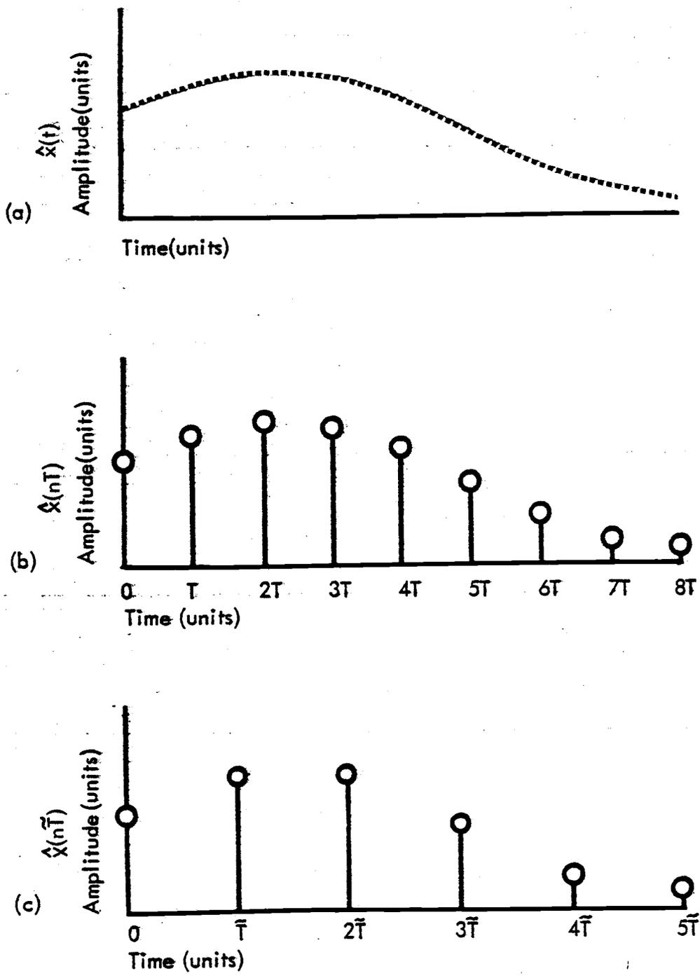
Fig. 1 (a) Graph of an analog signal. (b) Signal sampled every  $T$  units of time. (c) Signal sampled every  $\bar{T}$  units of time. At the instants in time indicated by circles the signal's amplitude is converted in to a form suitable for computer processing.
