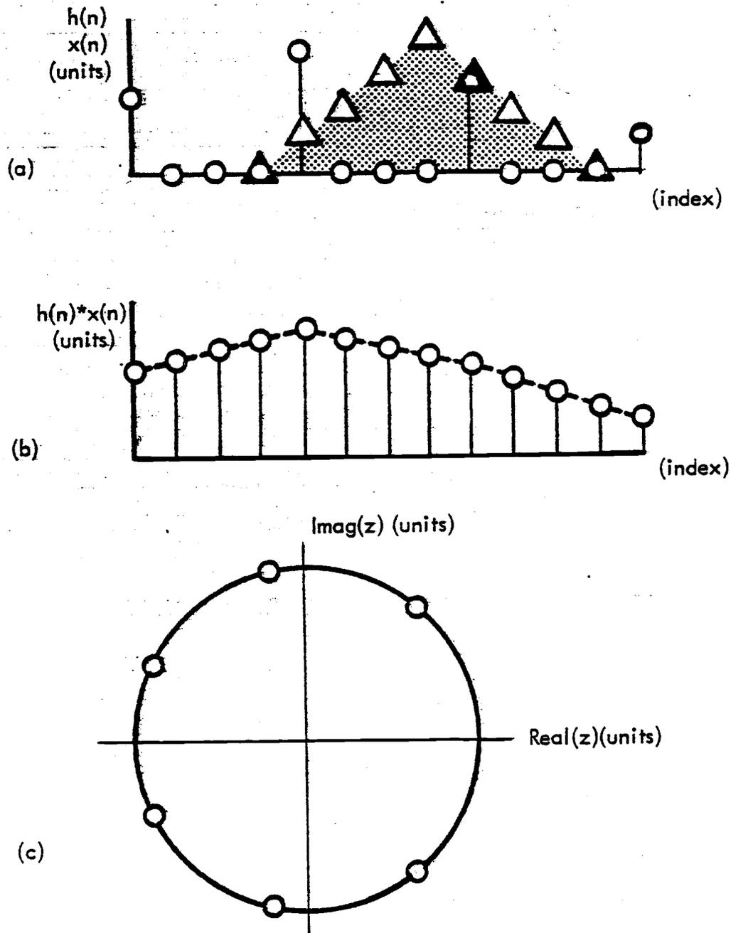
Fig. 13 (a) Interpolated sequence superimposed over a filter sequence. (b) Convolution of the interpolated sequence with the filter results in a linearly interpolated sequence. (c) Zero plot of the filter's z-transform.
