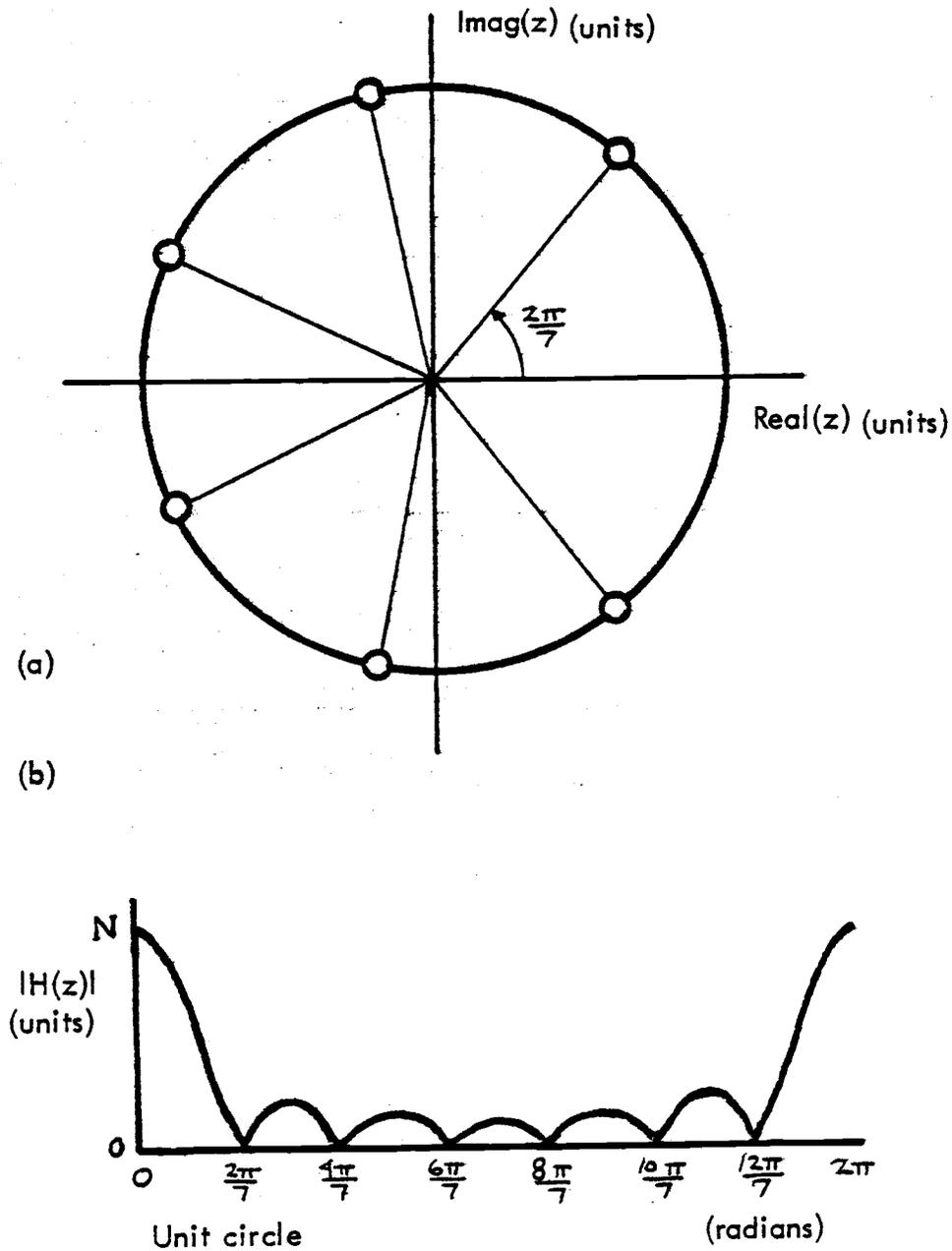
Fig. 3 (a) Unit circle plot and (b) Unit circle magnitude plot of the z-transform of the impulse response of an averaging filter where  $h(n) = 1$  for  $n = 0, 1, 2, 3, 4, 5,$  and  $6$  and  $h(n) = 0$  for all other values of  $n$ . Unit circle magnitude plot is the function  $|\sin(w7/2)/\sin(w/2)|$ .
