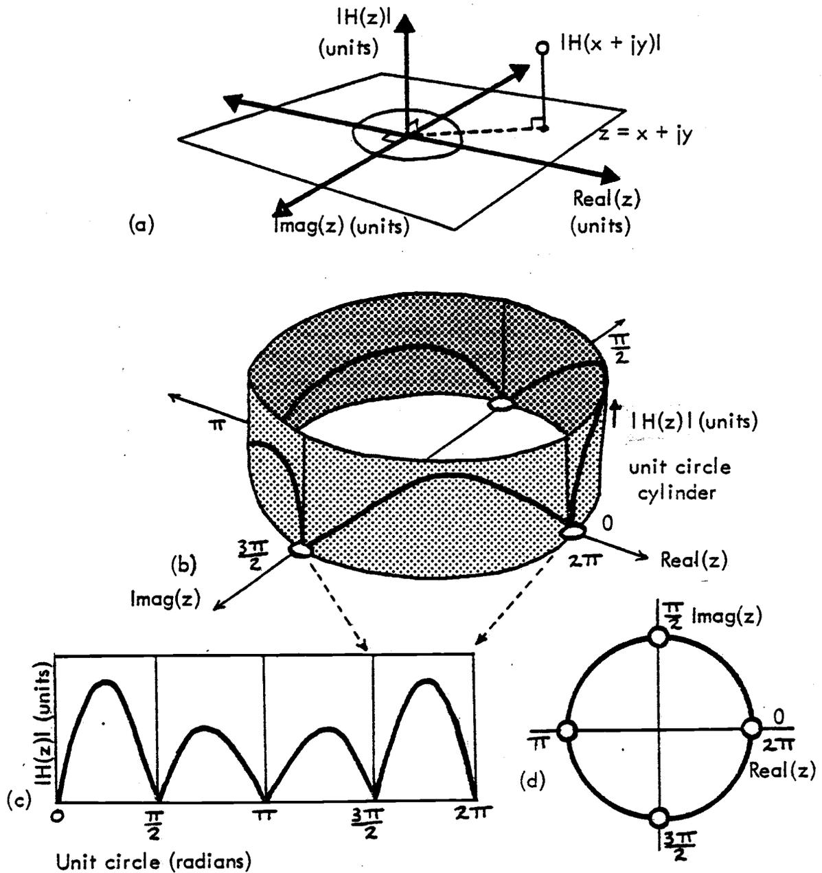
Fig. 2 Z-plane plotting conventions. (a) Three dimension plot of  $|H(z)|$  and the real and imaginary parts of  $z$ . (b)  $|H(z)|$  plotted on a cylindrical section of radius one. (c) Cylindrical plot projected on a flat surface. (d) Unit circle plot of values of  $z$  where  $|H(z)| = 0$ .
