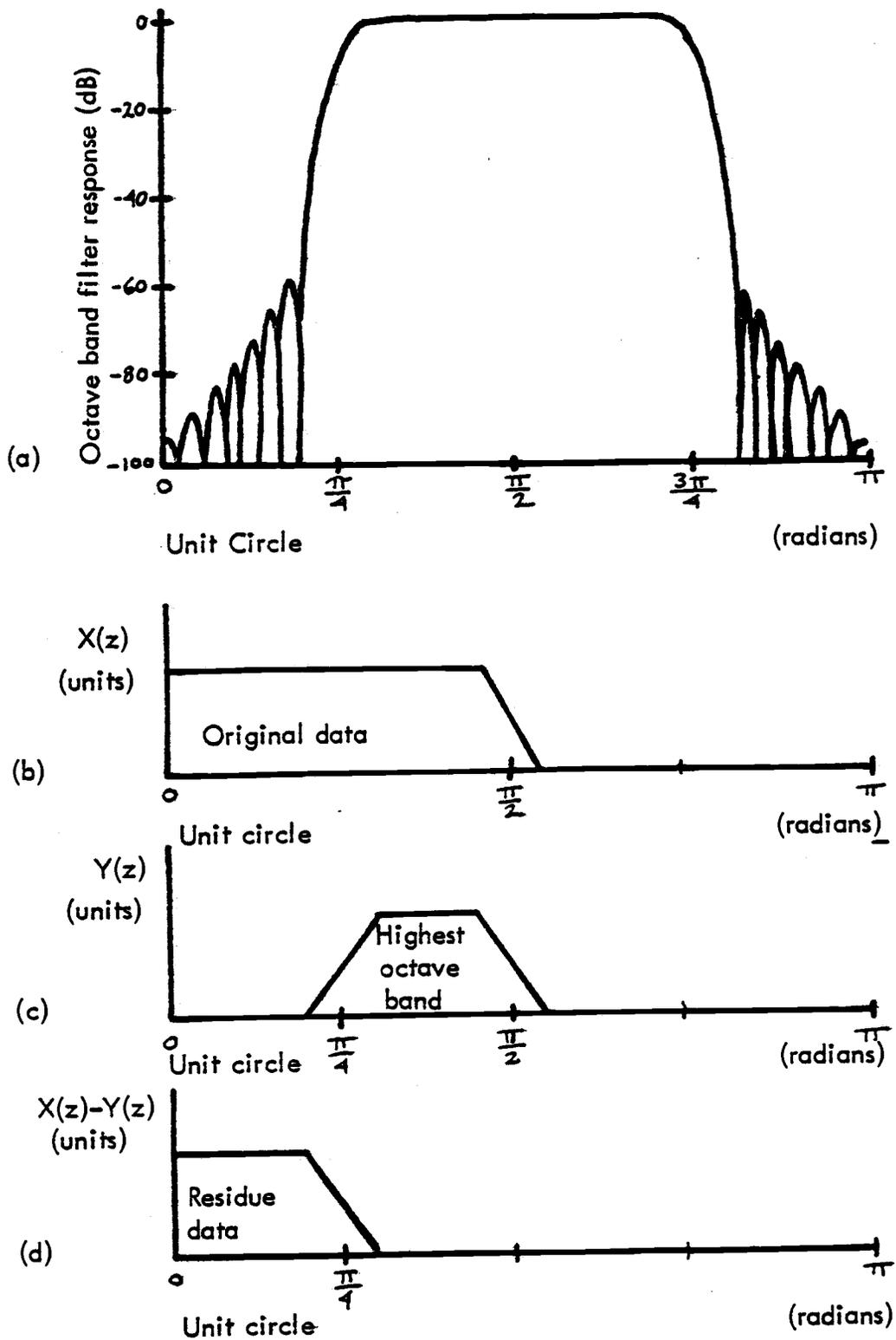
Fig. 14 (a) Typical response of an octave band filter. (b) Original data bandlimited to  $\pi/4$ . (c) Highest octave band after filtering  $X(z)$ . (d) Residue after subtraction. Resulting signal may be decimated by 2, and the filtering process repeated to yield the next octave band.
