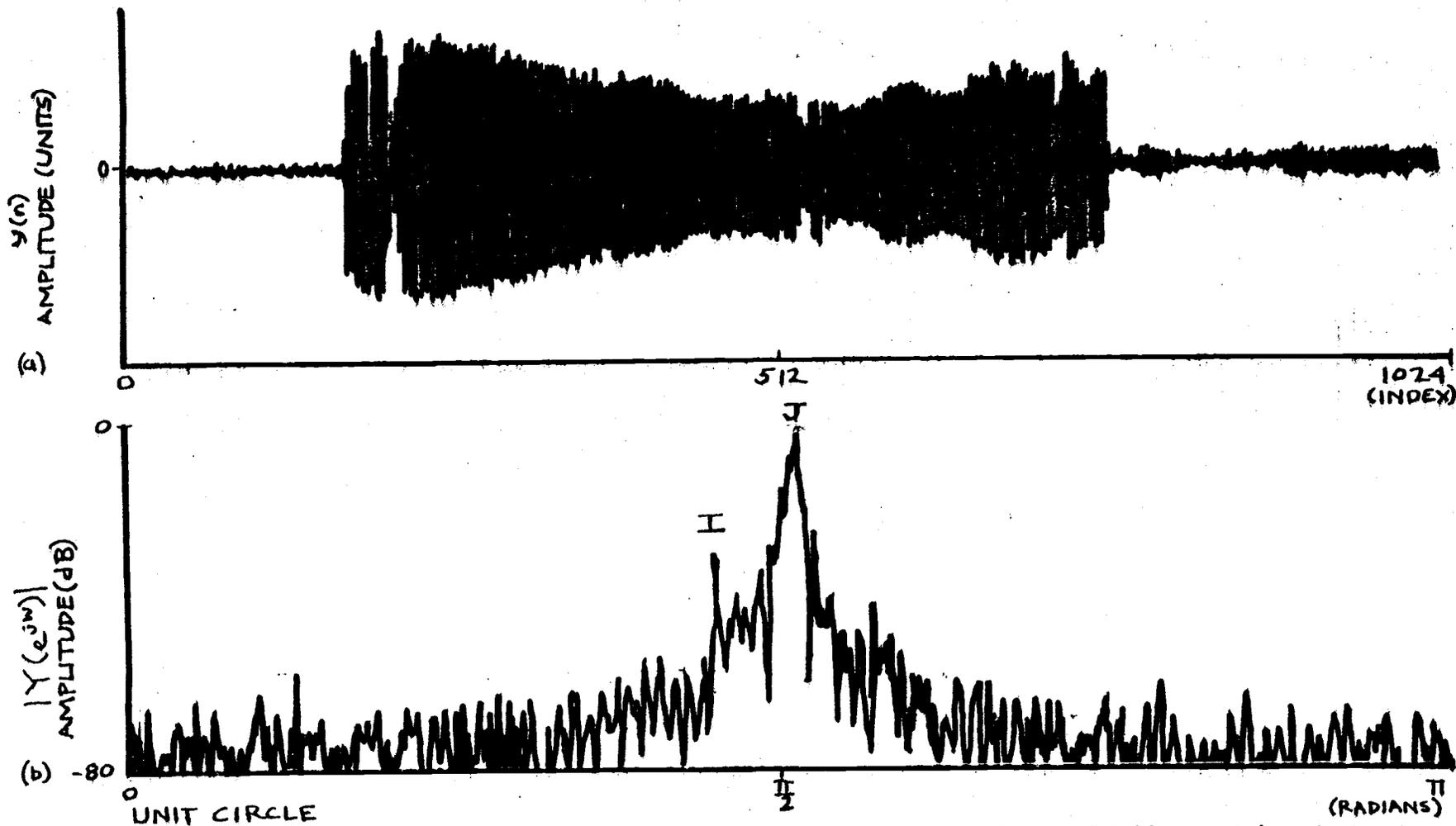
Fig. 12 (a) Sequence resulting after filtering the original sequence with a 128 point FIR filter and then decimating by 8. (b) Z-transform of sequence on the unit circle. Letters correspond to those in figure 9. The information in the region of interest has been preserved with a fewer number of samples.
