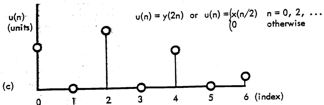
Fig. 5 (a) Original sequence  $x(n)$ . (b)  $x(n)$  interpolated by 4. Three zero values are inserted between each sample. (c)  $y(n)$  decimated by 2. Notice that this is equivalent to interpolating  $x(n)$  by 2.
