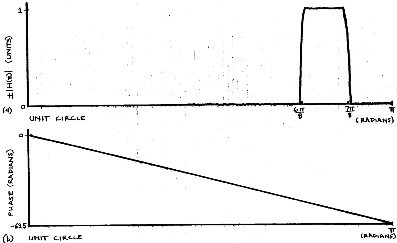
Fig. 11: (a) Magnitude response of 128 point FIR filter. (b) Linear phase response of filter. The magnitude function is plotted with both positive and negative values to achieve a linear phase plot. If the magnitude of  $H(z)$  were plotted, then the phase would change by  $\pi$  radians every time  $H(z)$  passes through a zero.
