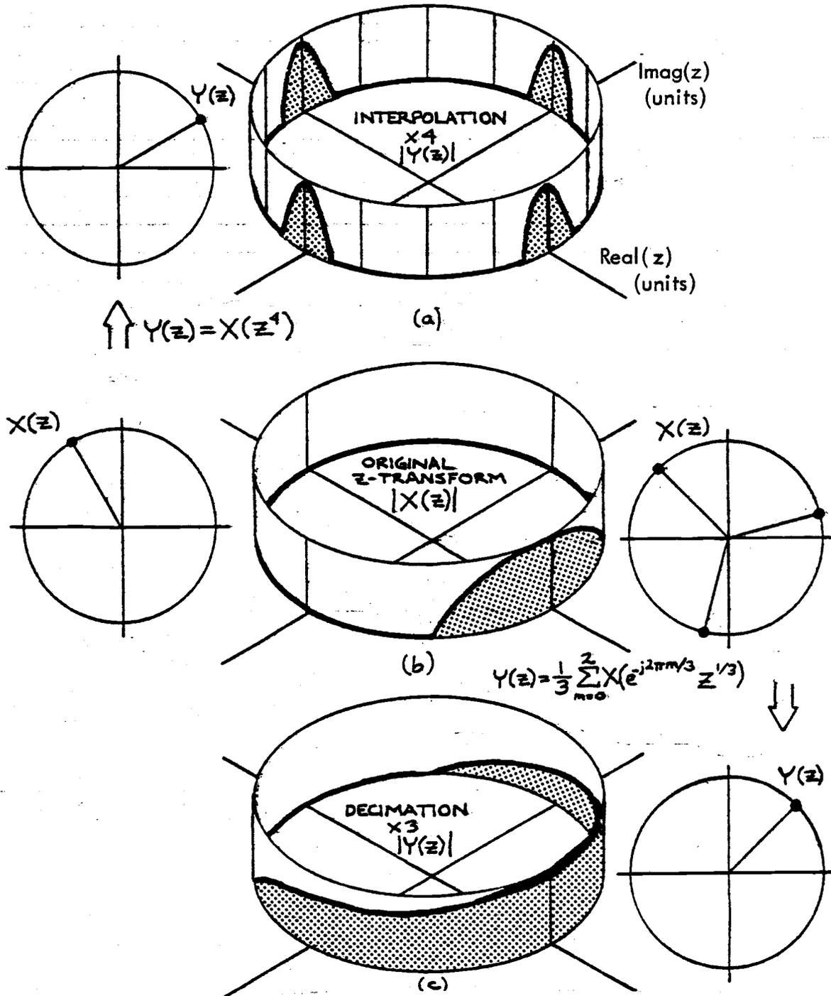
Fig. 6 (a) Sketch of the z-transform resulting from interpolating a sequence  $x(n)$  by 4. (b) Z-transform of the original sequence  $x(n)$ . (c) Sketch of the z-transform resulting from decimating  $x(n)$  by 3.
