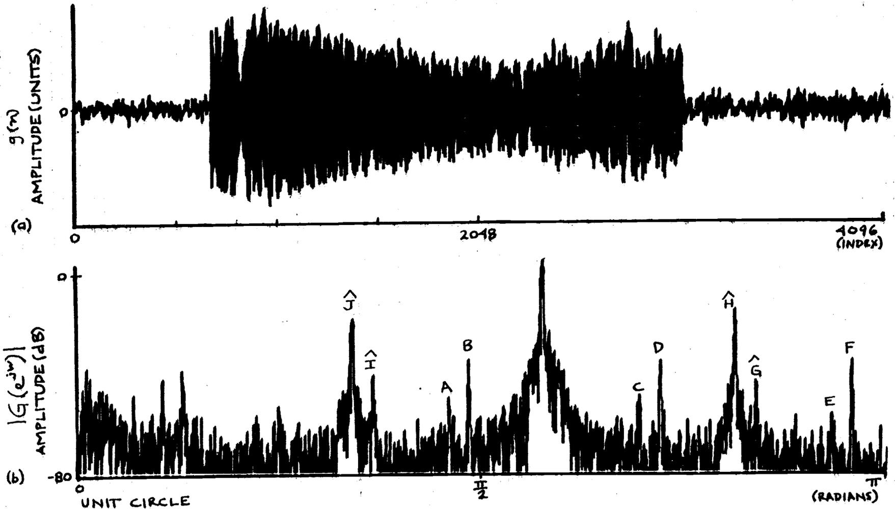
Fig. 10 (a) Original sequence decimated by 2. (b) Z-transform of decimated sequence on the unit circle. The components which summed due to aliasing are labeled with letters. Letters with hats are the same magnitude as the corresponding letter in Fig. 9.
