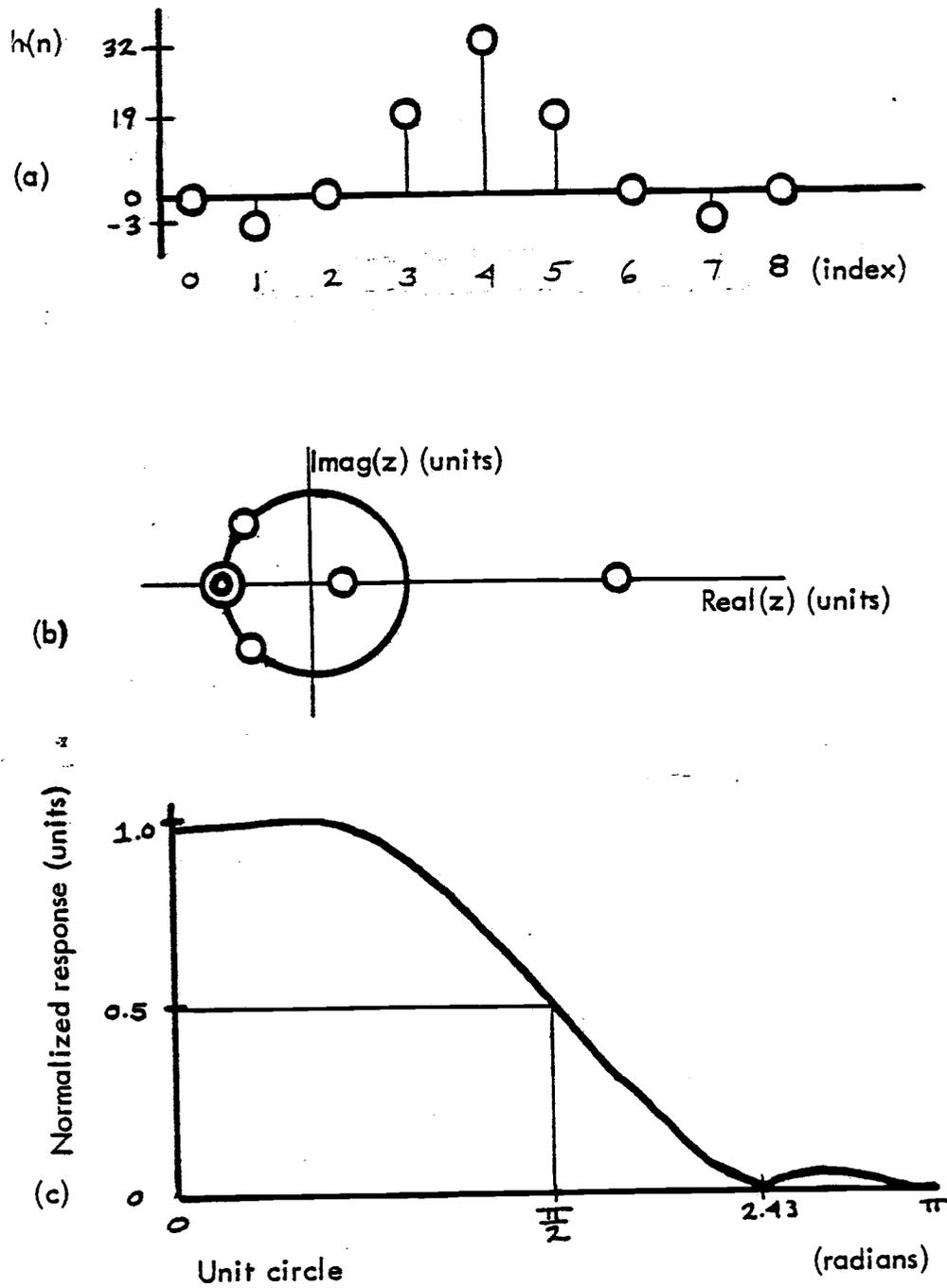
Fig. 15 (a) Nine-point half-band filter. (b) zero plot of half-band filter. (c) Unit circle magnitude plot of half-band filter.
