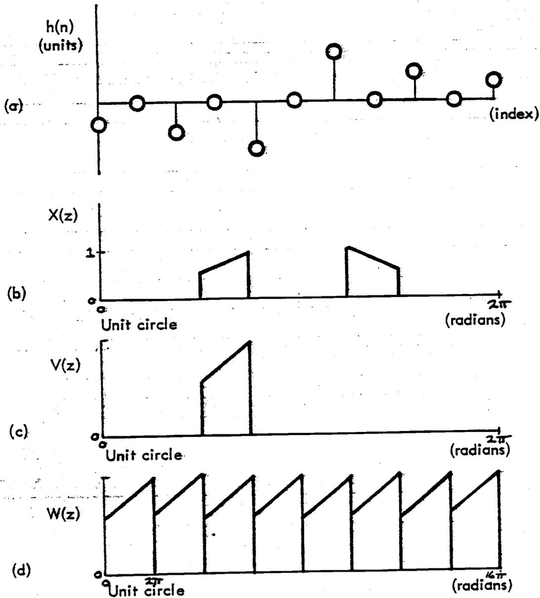
Fig. 16 (a) Typical Hilbert filter sequence. (b) Unit circle magnitude plot of a sequence. (c) Result of summing the sequence with its Hilbert filtered version. (d) Decimation of the sequence by 8.
