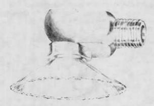
The side-entry hollow cone or "whirl-chamber" nozzle produces a very wide angle hollow cone spray pattern at very low pressures. It has a large opening and resists clogging. Because of the wide spray angle, the boom can be operated low, reducing drift. Spacing for double coverage and angling 15° to 45° to the rear is recommended for uniform application. These nozzles may be used in place of flat fan nozzle tips in broadcast applications.
