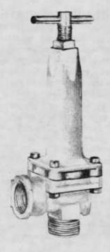
Unloader valves work like a spring-loaded bypass valve when the sprayer is operating. However, when the nozzles are shut down, they reduce strain on the pump by moving the overflow back into the tank at low pressure. These valves should be used on larger positive-displacement pumps (piston and diaphragm) to avoid damage to the pump or other system components when the nozzles are cut off.
