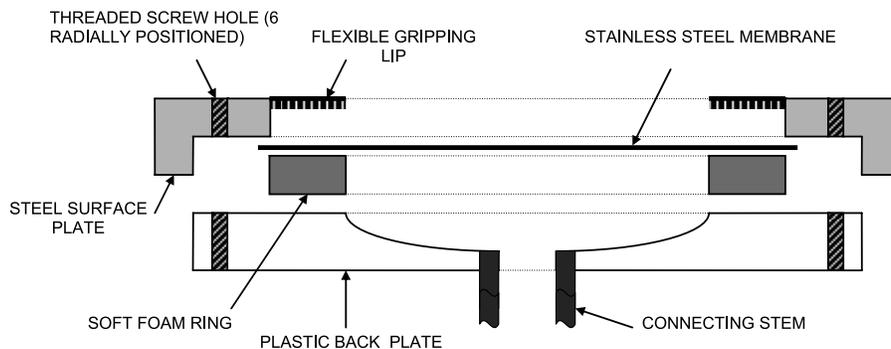
**Figure 2.** Base plate design showing screw assembly and serrated gripping lip. Note that the compression plate is shown prior to assembly. When assembled, the flexible gripping lip is in firm contact with the membrane, both pressing it against the rubber and holding it from slipping as it is tensioned. The unit used to generate the data shown has an overall diameter of 0.18 m, a contact diameter of 0.090 m, and a thickness of the entire device of 0.028 m.
