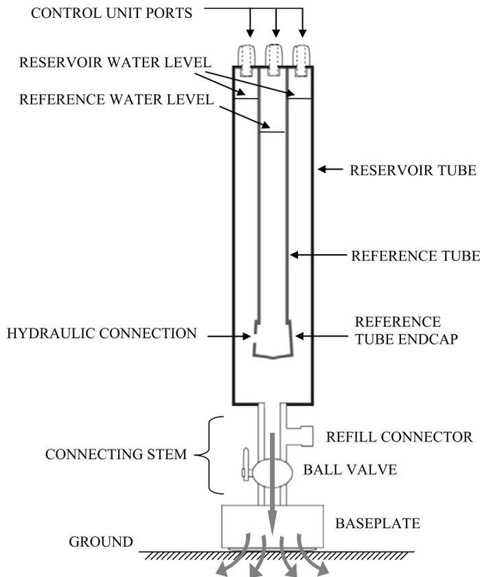
**Figure 1.** Infiltrometer components. The pneumatic valves are attached to the control ports either directly or via tubing. The contact area of the screen employed here was a circle of 8.5 cm diameter.
