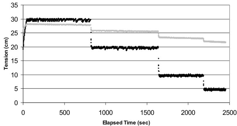
**Figure 3.** Test results from experiment carried out in a 50–1 drum packed with Willakenzie silt-loam soil: negative pressure head (tension in cm) over time at membrane (black diamonds) and 0.2 times the reservoir head space pressure (gray diamonds), from which the delivered volume is computed. Data points are separated by 1 s. The rate of infiltration is computed from the slope of the reservoir pressure via the density of water and surface area of water in the reservoir.
