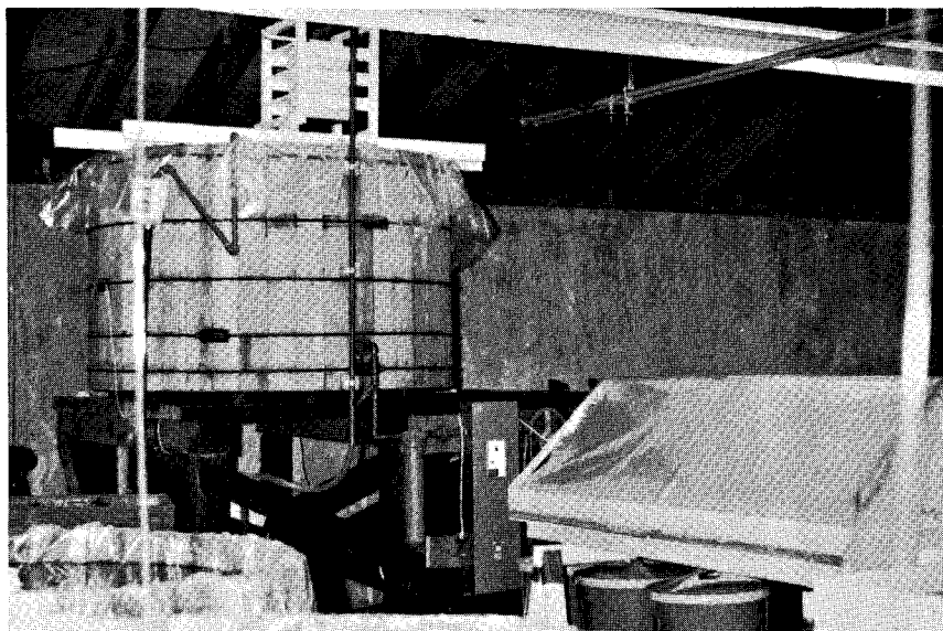
Figure 2. The Larval Rearing System Showing the Pre-system Filter, Head Tank, 5 Micron Filter, Ultra-violet Unit, Incubating Enclosure and Sump.
