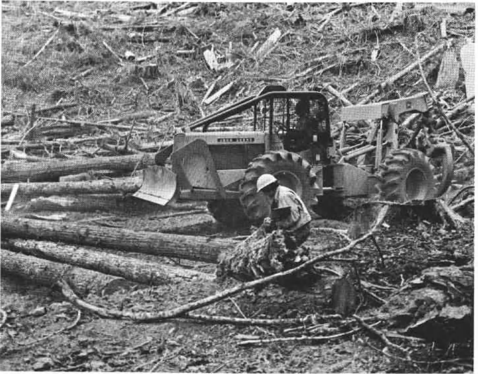
Figure 3. A grapple-equipped skidder was used on the balloon operations to move logs from the unhooking area to the loader. At short yarding distances, the unhooking area occasionally became overcrowded with logs and the yarder was forced to wait until the area had been cleared. In the foreground of this photograph is one of the time-study crewmen, shown measuring log volume.
