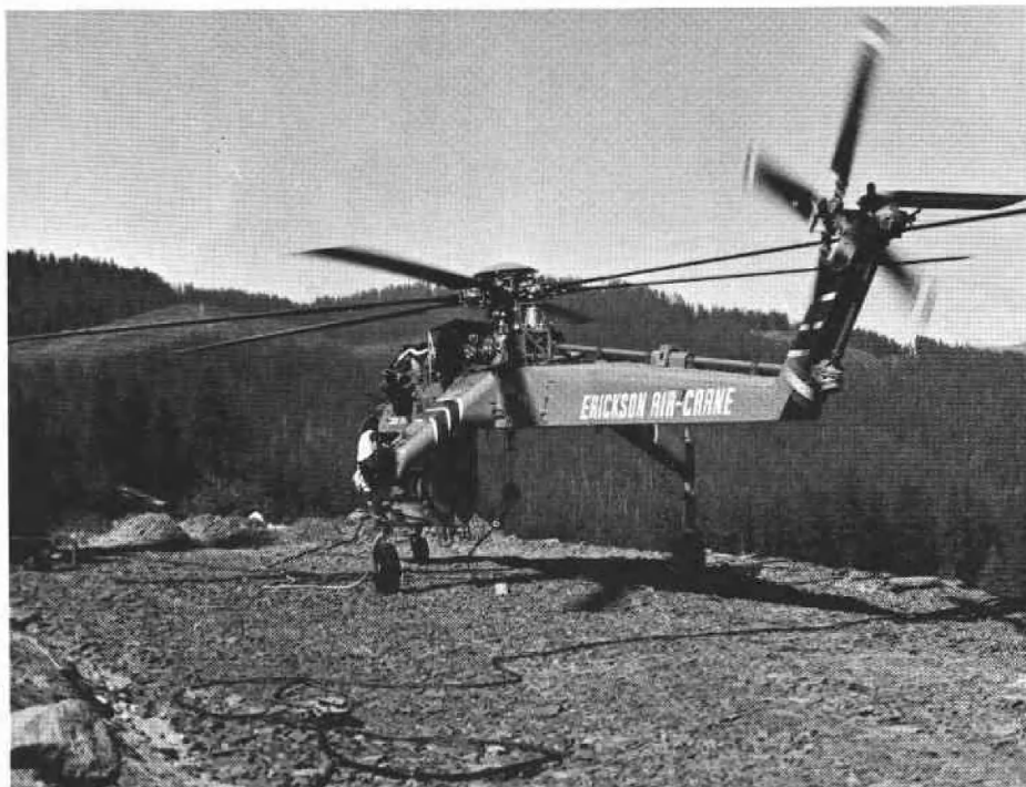
Figure 1. The Sikorsky Skycrane helicopter on the refueling pad. The need for frequent refueling stops proved to be the greatest single cause of delay on the two helicopter operations in this study.
