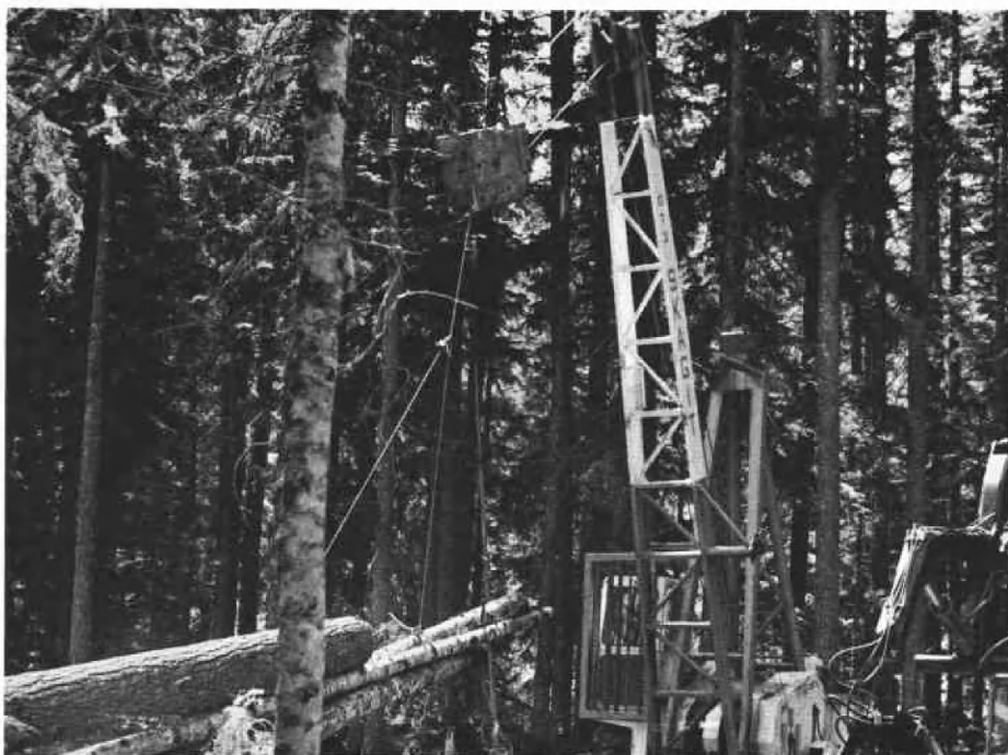
Figure 2. A partial-cut silvicultural prescription on the running skyline operation necessitated the use of a carriage capable of lateral yarding. The high frequency of repair and maintenance delays on this operation was largely attributed to problems with this complex carriage.
