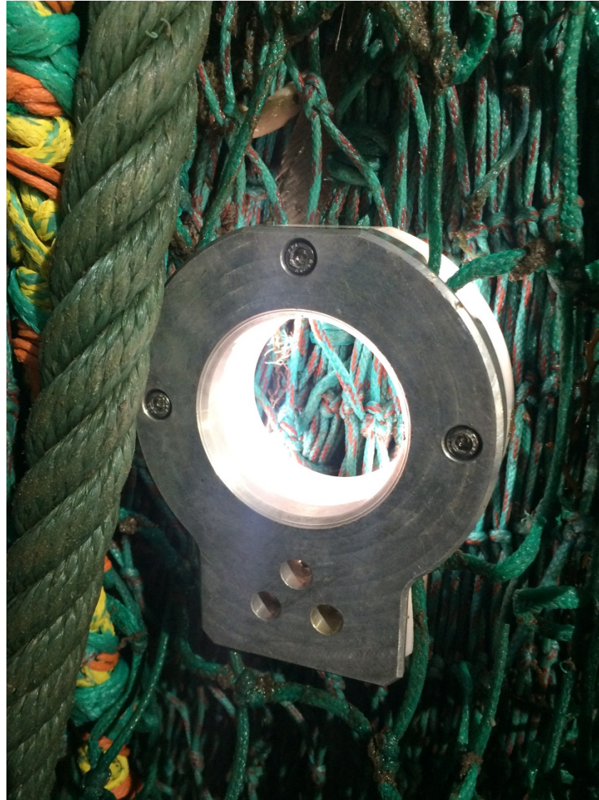
The Trawligh Gear, 90mm aperture Light rings (x6) – Bright LEDs bolted into the Square mesh panel on the starboard side trawl
