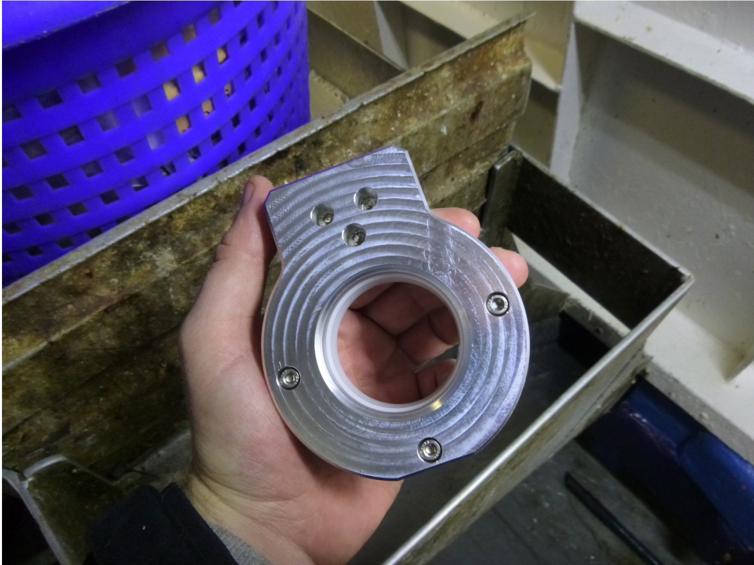
The Trawligh Gear, 90mm aperture Light rings (x6) – Bright LEDs bolted into the Square mesh panel on the starboard side trawl
