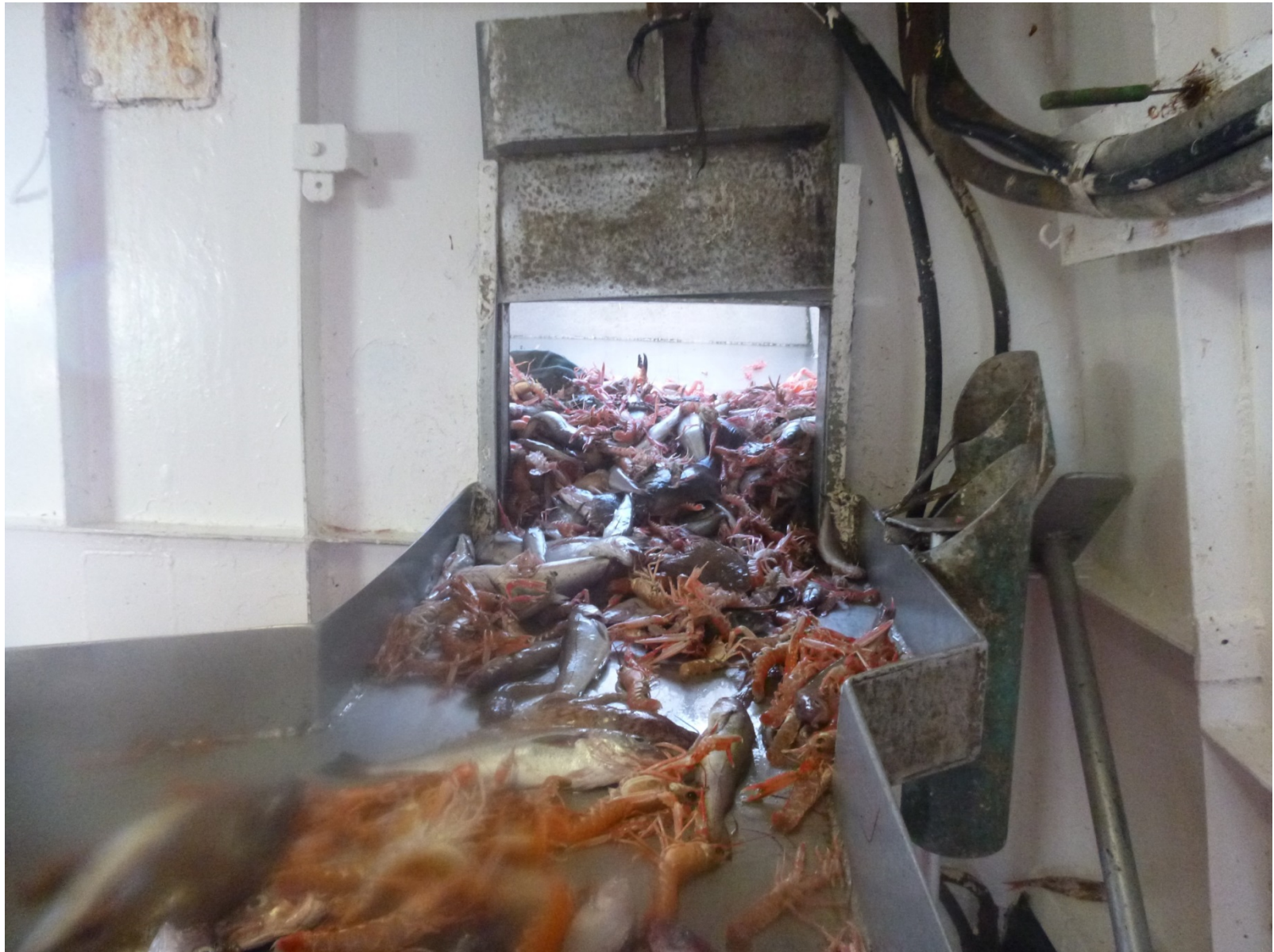
The Catch being released from the cod end of the net into the hopper on the open deck and then channelled through into the sorting table under the shelter deck
