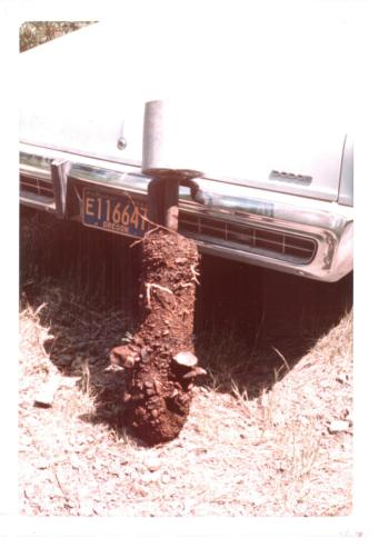
Figure 2: Frozen core after extraction from the streambed.
