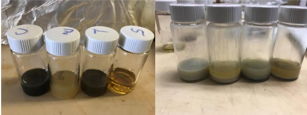
**Figure 2.5 Photos of fresh made inks (Left) and ink after 24 hours (Right)**
