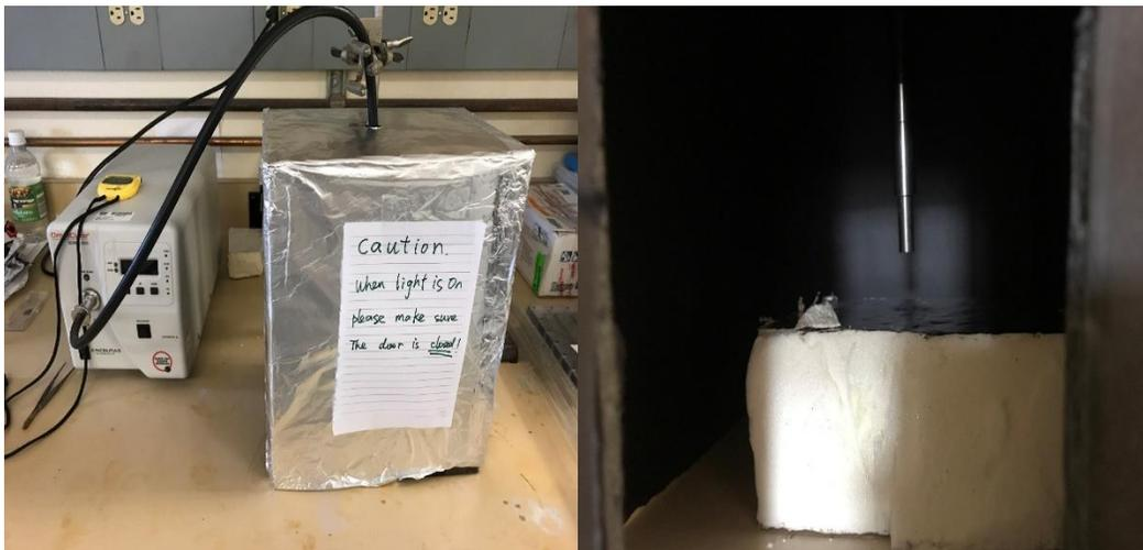
**Figure 2.11 Outside (Left) and inside (Right) view of UV curing system setup**
