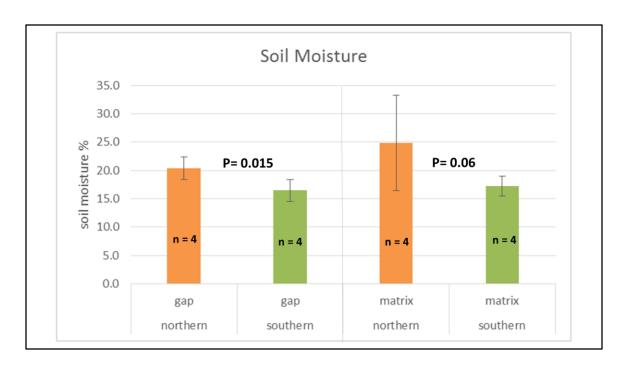
The class collected and analyzed soil samples from the two locations. Preliminary data from just 4 sites in each section suggests that soil moisture is higher in the northern section than it is in the southern section. This is consistent with the lower mortality rates from beetle attack that we have seen in the northern part of the preserve.
