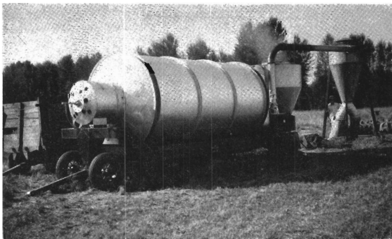
Figure 4. Portable rotary-drum dehydrator being tested on alfalfa in Linn County.
