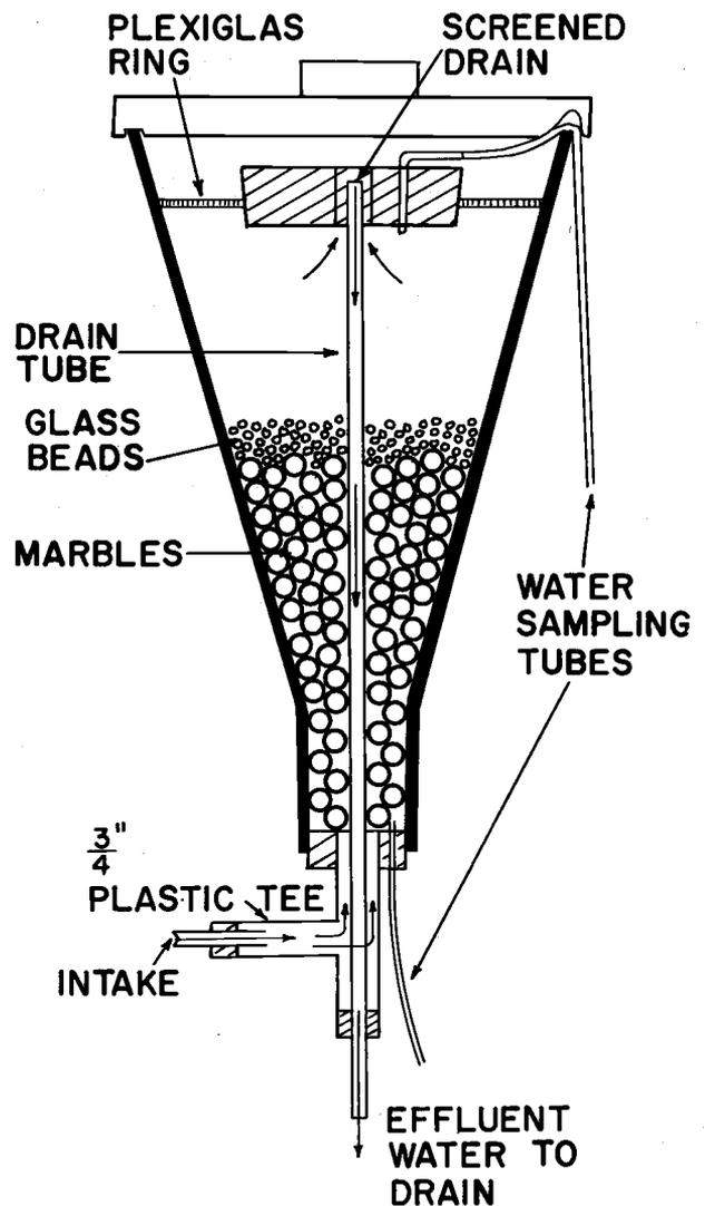
FIGURE 2. One of six experimental chambers used to expose steelhead trout eggs and alevins to dieldrin in Experiment 2. The eggs were placed in a single layer directly on the glass beads.
