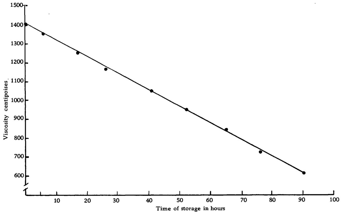
Figure 4. The viscosity of strawberry slurry stored at 72° F as a function of the storage time.
