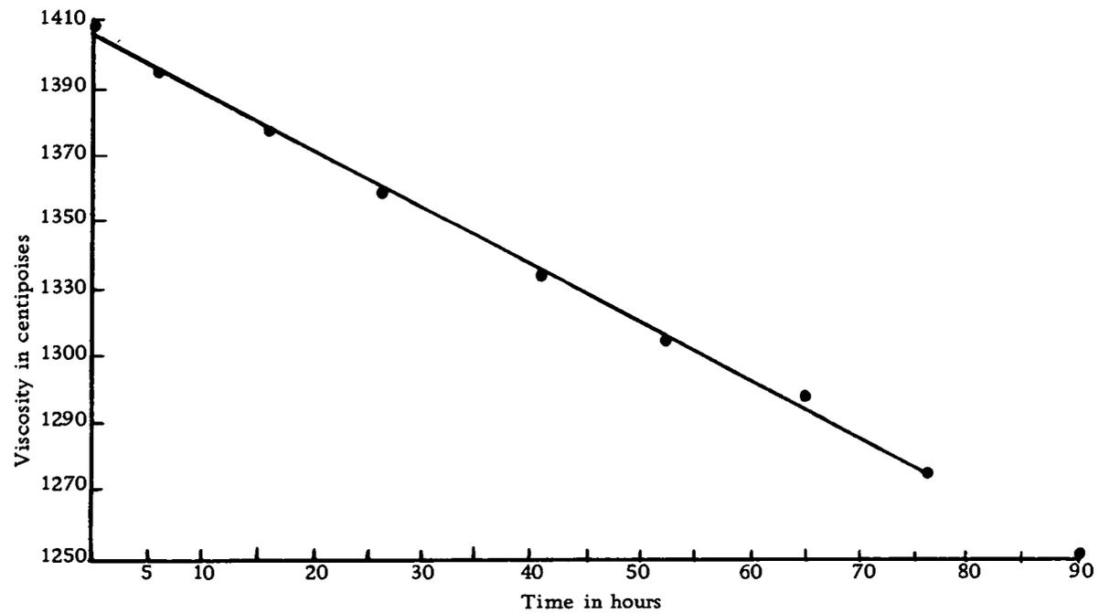
Figure 5. The viscosity of strawberry slurry stored at 34°F as a function of the storage time.
