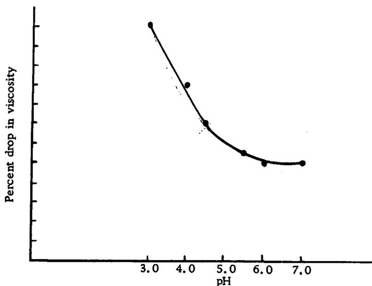
Figure 12. Percentage drop in viscosity of sodium pectate solutions at different pH and temperature 30°C.
