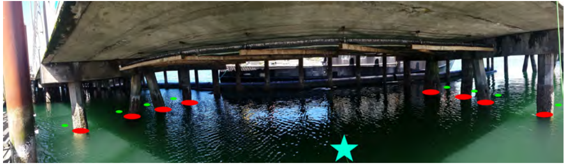
Figure 3.6: Oregon State University Ship Operations Pier in Newport, Oregon used for field trials. The robot must visit each of the inspection locations indicated by green dots while avoiding becoming entangled by the wharf pilings shown as red circles. The robot is deployed from the base station located at the blue star.
