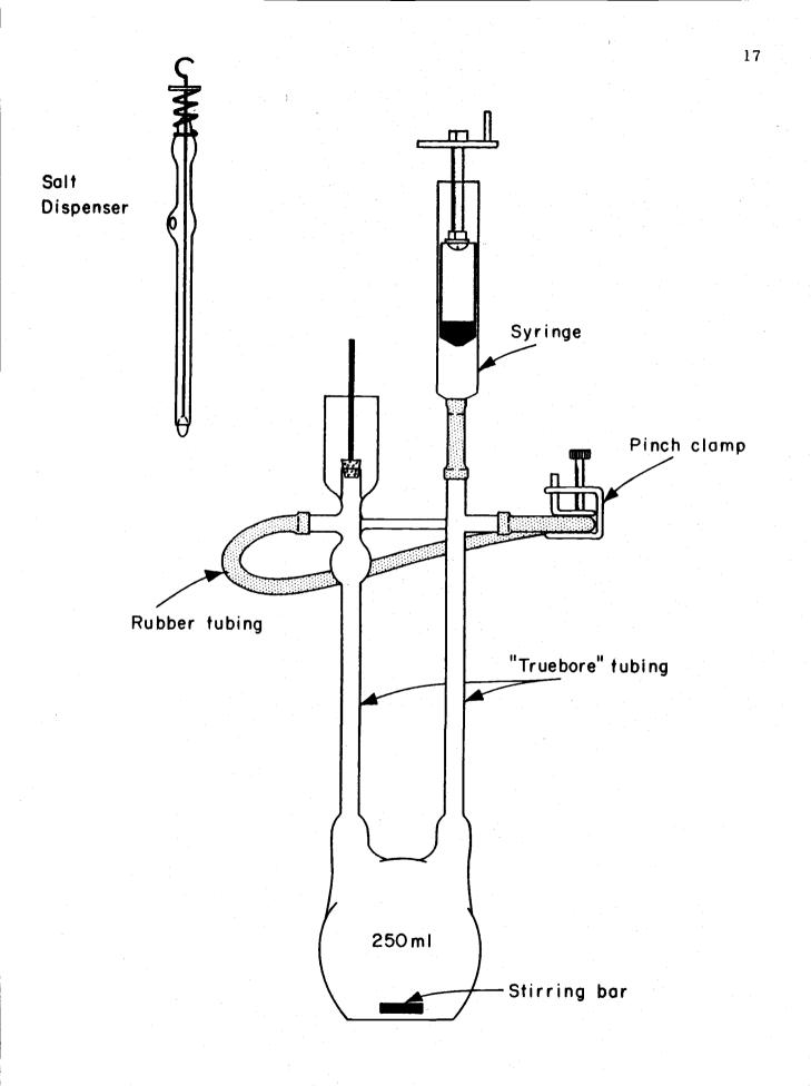
Figure 3. Dilatometer.
