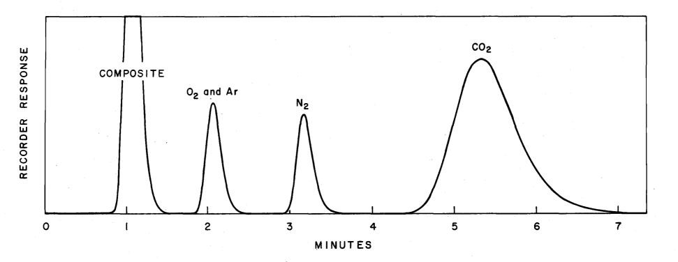
Figure 1. Gas chromatogram of oxygen (plus argon), nitrogen, and total carbon dioxide.
