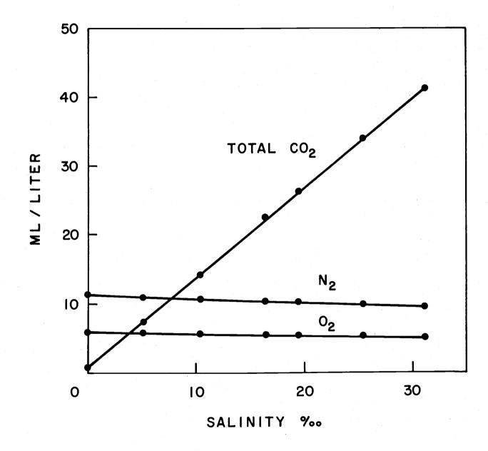
Figure 2. Oxygen, nitrogen and total carbon dioxide in sea water as a function of salinity. The method originally proposed for determining partial molar volumes by changes in density has been improved. A special dilatometer (Figure 3) was developed for the direct determination of the volume change due to salt addition. A constant temperature bath for the system has been constructed, and initial tests of the equipment have been satisfactory.
