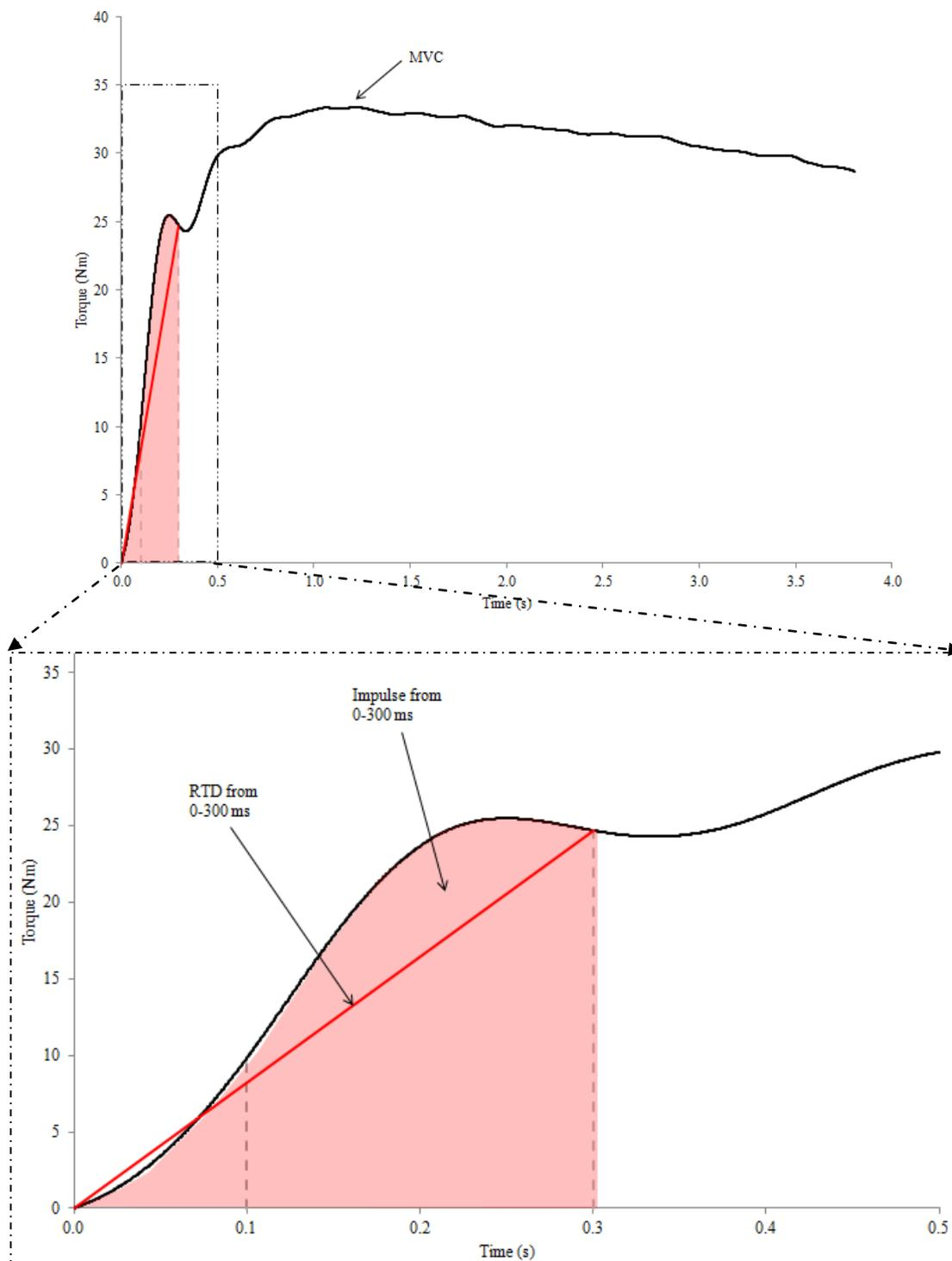
**Figure 5:** Representative torque-time curve. The upper panel shows the torque recorded across the full length of the trial. This includes the maximum voluntary contraction (MVC). The lower panel is an expansion of the initial 500 ms of the contraction. Contractile impulse is represented by the shaded area and rate of torque development (RTD) by the solid line for the 0-300 ms time period.
