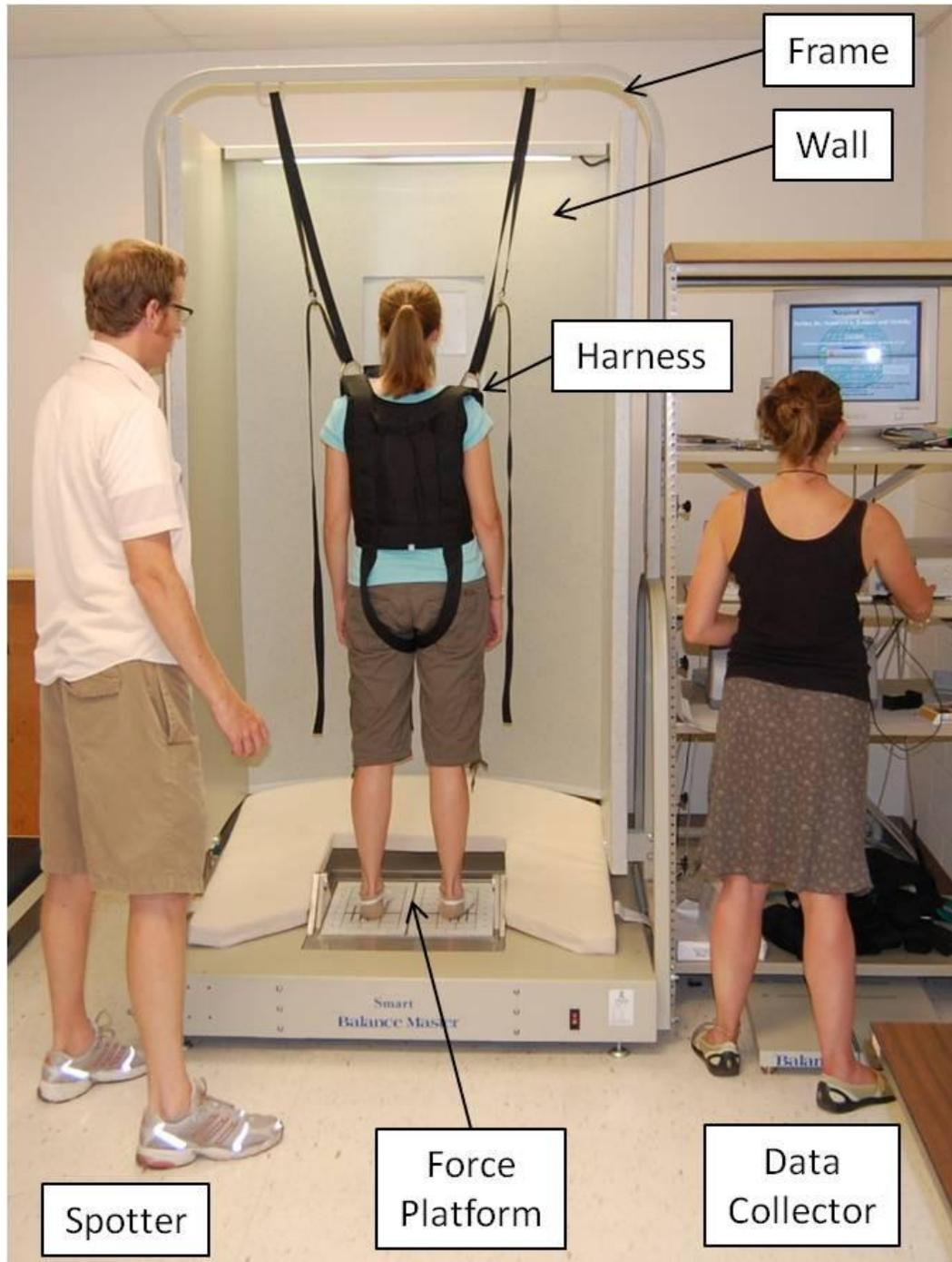
**Figure 1:** Sensory Organization Test setup. The participant removed her shoes and was positioned in a safety harness that attached securely to the frame. Her feet were properly aligned on the force platform. The force platform measured the participant's center of gravity sway. Some test conditions included sway of the force platform and/or the wall.
