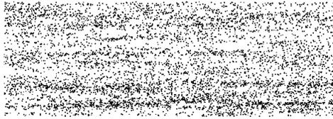
Figure 6.43: *Instantaneous particle structures in the near wall region ( $0 < y^+ < 4$ ) for the  $m = 0.01$  case using volumetric coupling and neglecting the effects of collisions, with  $St = 0.89$ .*
