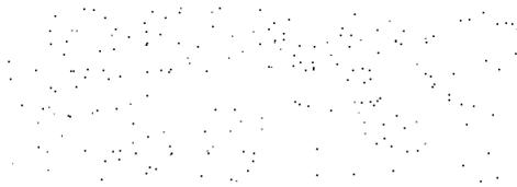
Figure 6.47: *Instantaneous particle structures in the near wall region ( $0 < y^+ < 4$ ) for the  $m = 0.2$  case using two-way coupling and neglecting the effects of collisions, with  $St = 70$ .*
