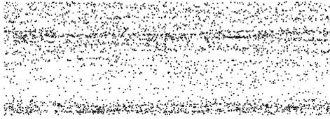
Figure 6.45: *Instantaneous particle structures in the near wall region ( $0 < y^+ < 4$ ) for the  $m = 0.2$  case using two-way coupling and neglecting the effects of collisions, with  $St = 10$ .*
