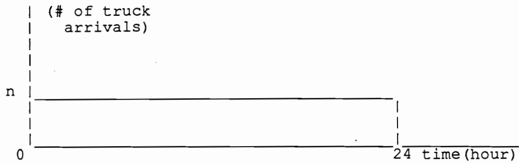
Figure 2. Desirable distribution of truck arrivals for 24 hour per day operation with equal crew size on each shift.
