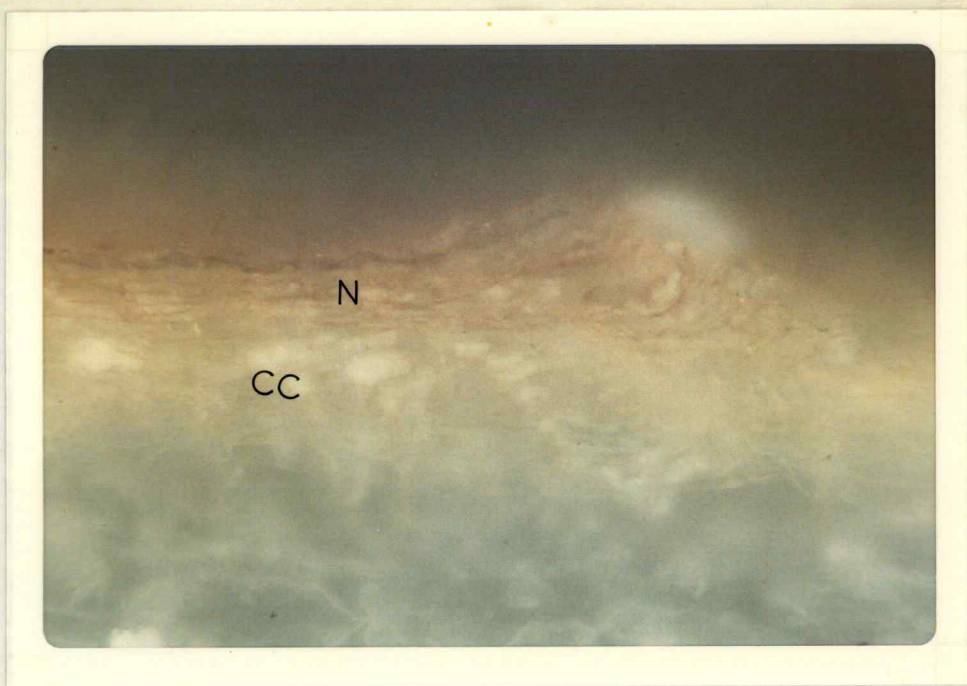
Figure 27 - Cross Section of Cork Showing Stained Cell Walls of Phelloid Cells (Net)
