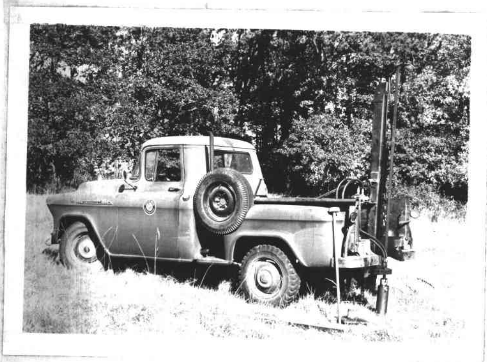
Fig. 7a. - Hydraulic coring rig used to extract soil cores for root distribution study.
