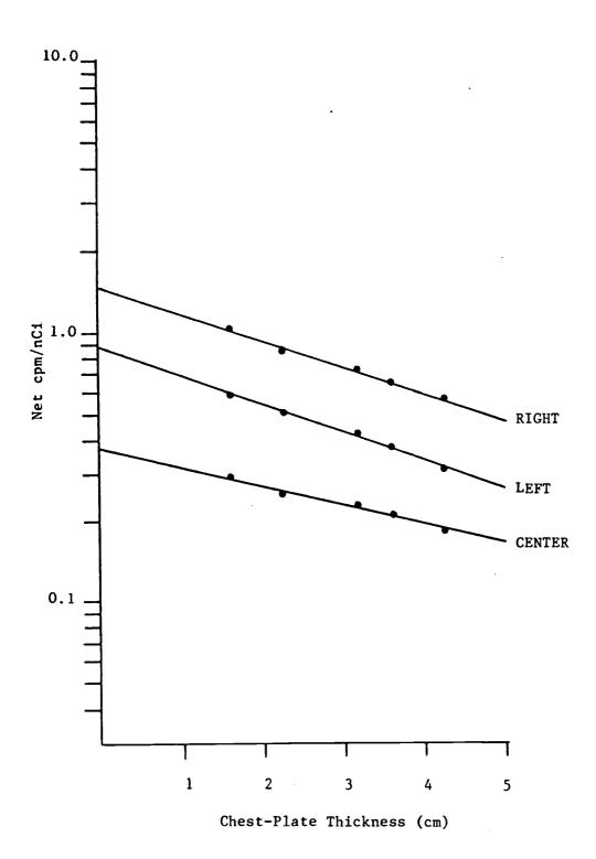
Figure 14. Phantom calibration data curves with the 13/87 chest-plates and the americium-241 (2200 nCi) TBLN point source.
