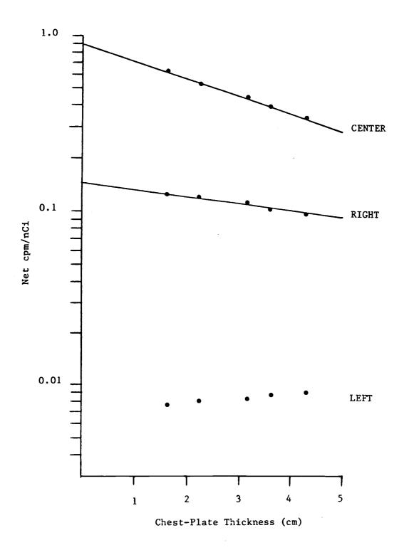
Figure 15. Phantom calibration data curves with the 50/50 chest-plates and the americium-241 (2200 nCi) TBLN point source.
