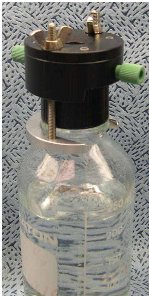
Figure 3.6 Photograph of the removable septum cap on a septum bottle.
