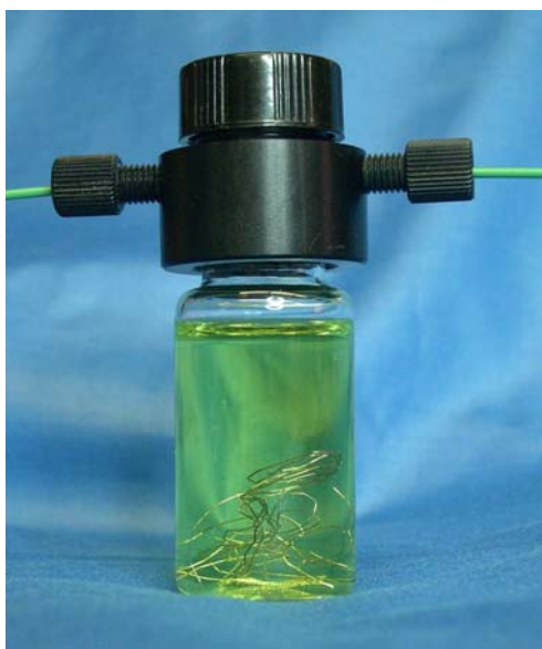
Figure 4.3 Photograph of reduced indigo carmine stock in a double-septum vial. The vial screw cap has a female threaded bottom and a male threaded top (22-400 GPI size for both). The gap between two septa (20-mm butyl rubber septa from Agilent Tech.) was continuously purged with N_2 .
