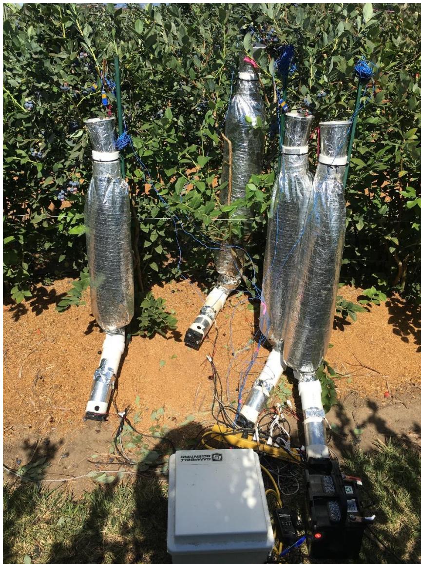
Fig. 2.1. A forced-convection unit for heating blueberry clusters in the field.
