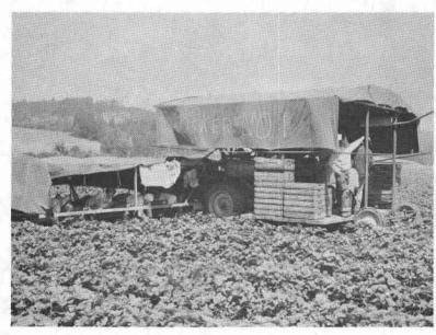
Figure 2. This ten-row personnel carrier was built on a used, self-propelled grain combine frame.
