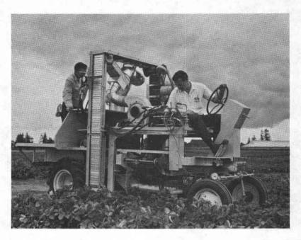
Figure 9. A full-row, self-propelled strawberry harvester was field tested by Oregon State University in 1968.
