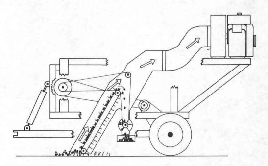
Figure 6. The operation of the University of Arkansas harvester is shown schematically (23).
