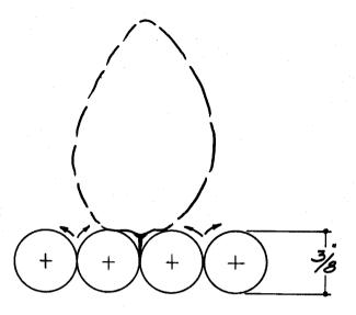
Figure 11. Counter-rotating rubber-covered rolls.
