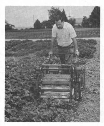
Figure 8. Compressed air is used to lift the strawberries off the ground in the operation of the harvester developed at the University of Guelph, Guelph, Ontario, Canada. [Ontario Department of Agriculture and Food photograph courtesy of Harold A. Hughes (25)].
