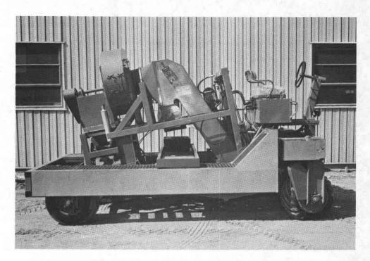
Figure 7. A production prototype of the University of Arkansas strawberry harvester has been built and tested by Blueberry Equipment, Inc. of South Haven, Michigan. [Photograph courtesy of Donald B. Cunningham (8)].
