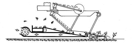
Figure 4. A side view of the Iowa State University harvester shows how air is used to aid in conveying the harvested fruit and in removing leaves. [Drawing courtesy of Graeme R. Quick (42)].
