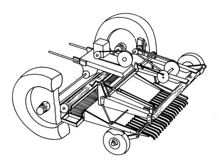
Figure 3. The strawberry harvesting device under development at Iowa State University features a row of oscillating fingers. [Drawing courtesy of Graeme R. Quick, (42)].
