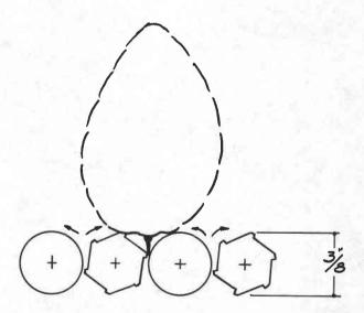
Figure 10. Serrated metal rolls matched against counter-rotating rubber-covered rolls.
