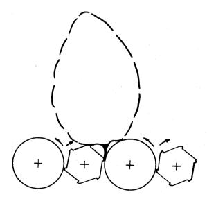
Figure 12. Serrated metal rolls matched with larger diameter rubber-covered rolls to give better tumbling action.
