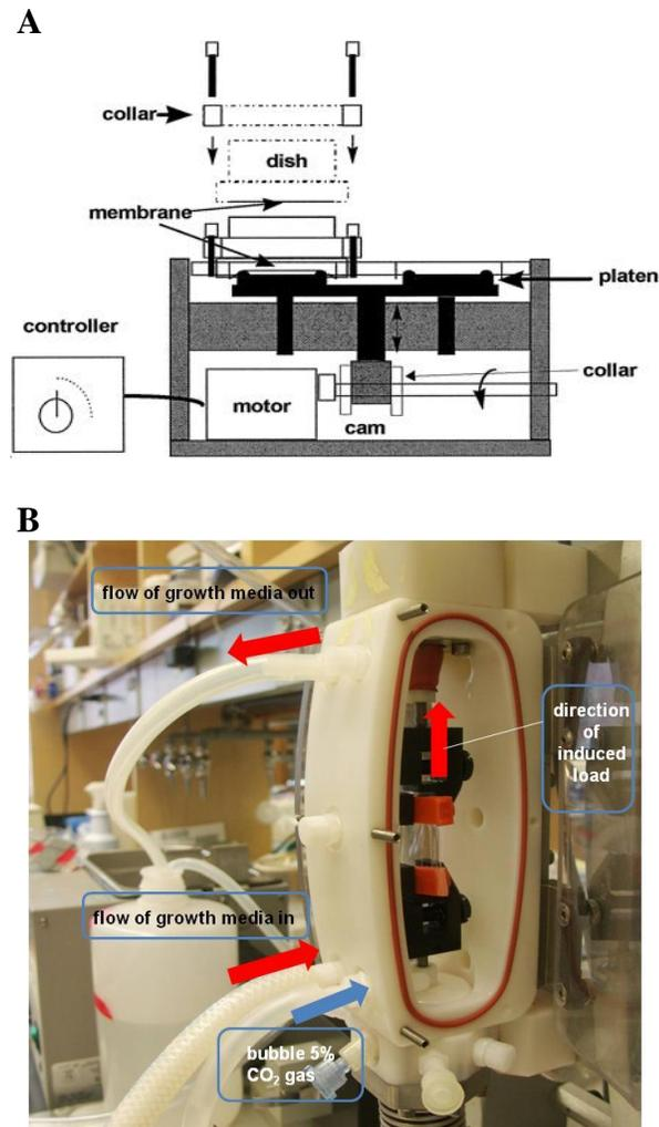
**Figure 2.** (A) Diagram of biaxial loading device similar to loading device used in this experiment [27], (B) View of BioDynamic test device used for uniaxial loading. Cell culture medium is flowed through test device with a 5% CO<sub>2</sub> bubbler to pH balance growth media.
