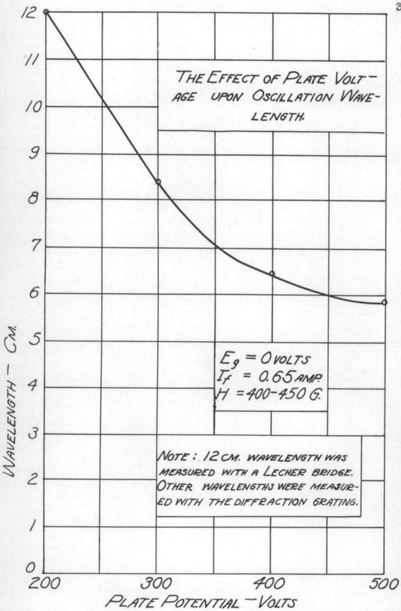
on the wavelength of the oscillations produced by the tube. There is a very striking similarity between this curve and a curve showing the effect of grid voltage on the wavelength of a Barkhausen-Kurz oscillator. This similarity is due to the similarity of mechanism of oscillation between the two different types of oscillator.
