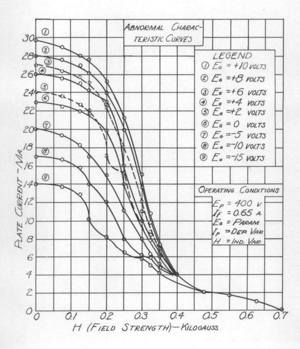
from zero to the point at which it prevented electrons from reaching the plate (cut-off).
