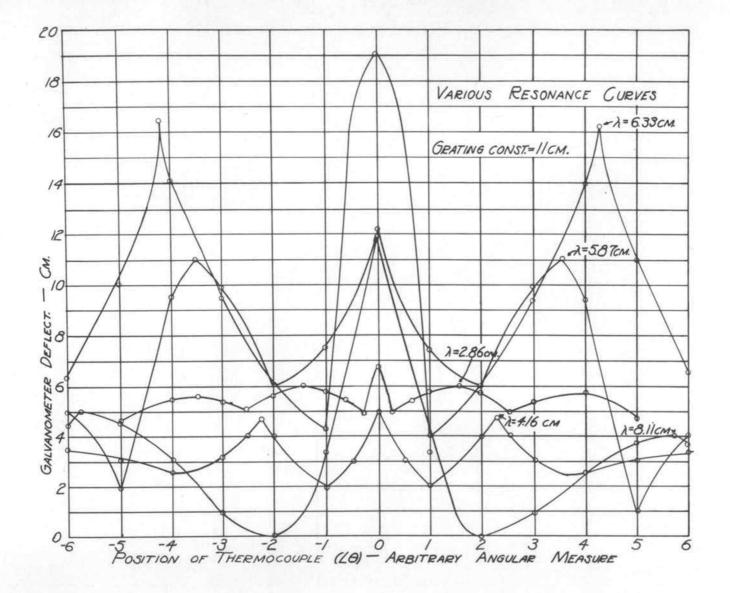
moved further in the same direction (counter clockwise) until the third order spectrum peak was passed, after which the thermocouple arm was moved back in a clockwise direction to the position of central maximum. Galvanometer readings were taken at each step. This procedure allowed every point to be checked twice during a run and each run was duplicated at some other time to check the results.
