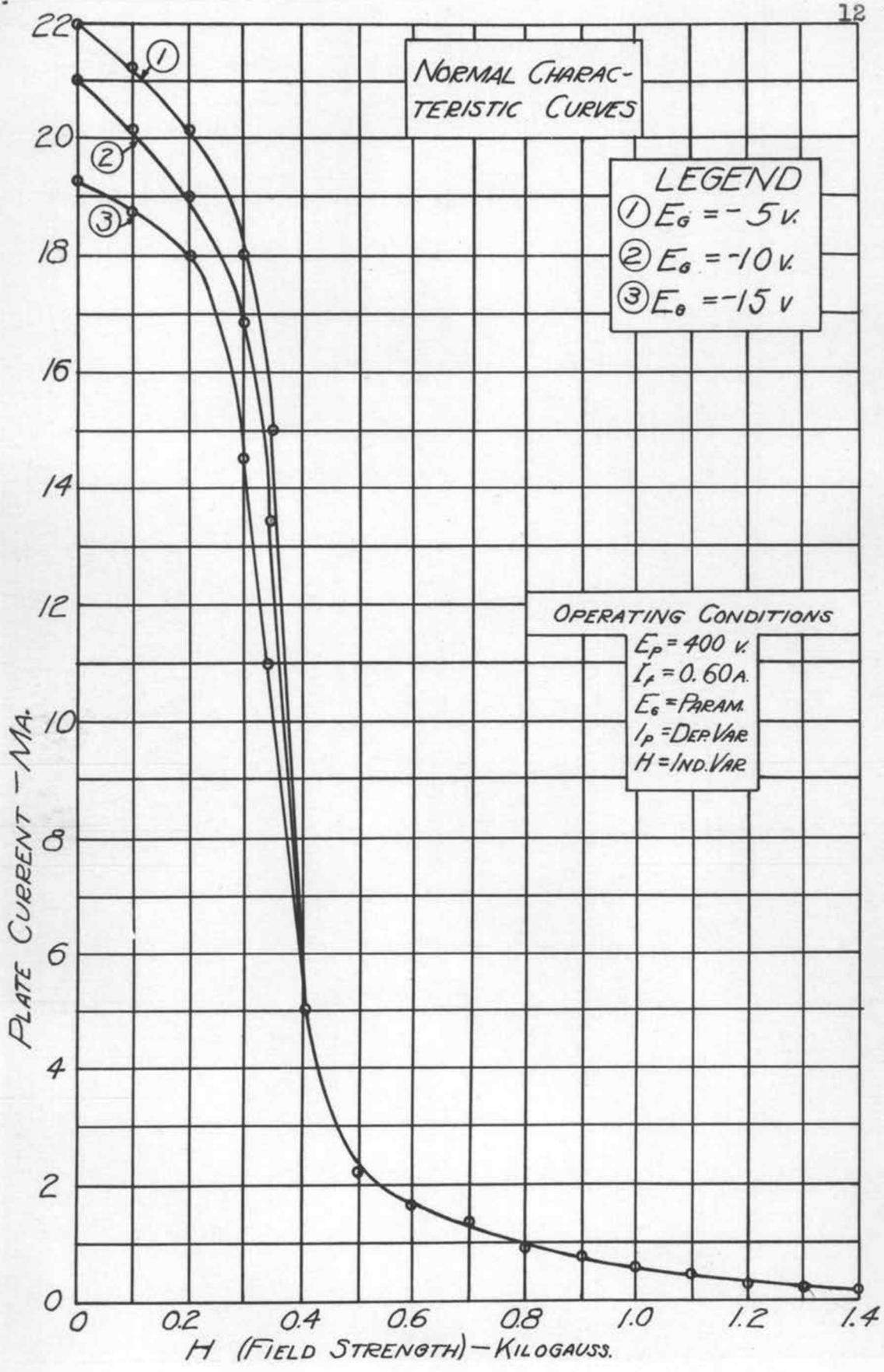
from zero to the point at which it prevented electrons from reaching the plate (cut-off).
