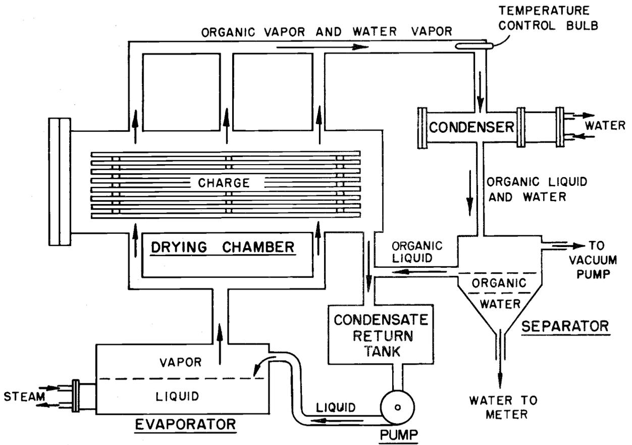
FIGURE 1. FLOW DIAGRAM OF VAPOR-DRYING PROCESS
