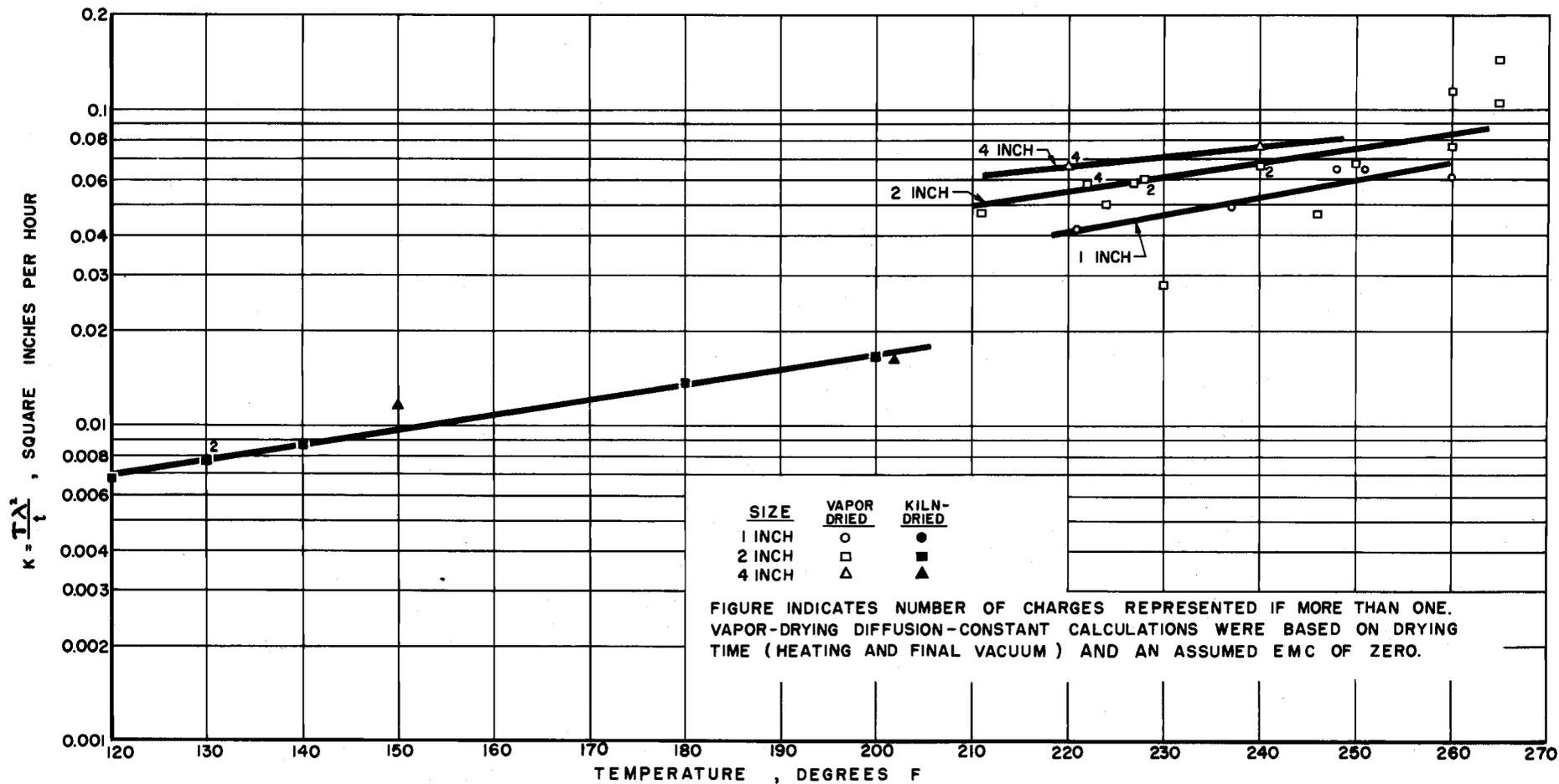
FIGURE 2. TEMPERATURE AND DRYING-DIFFUSION-CONSTANT RELATIONSHIP FOR DOUGLAS-FIR LUMBER.
