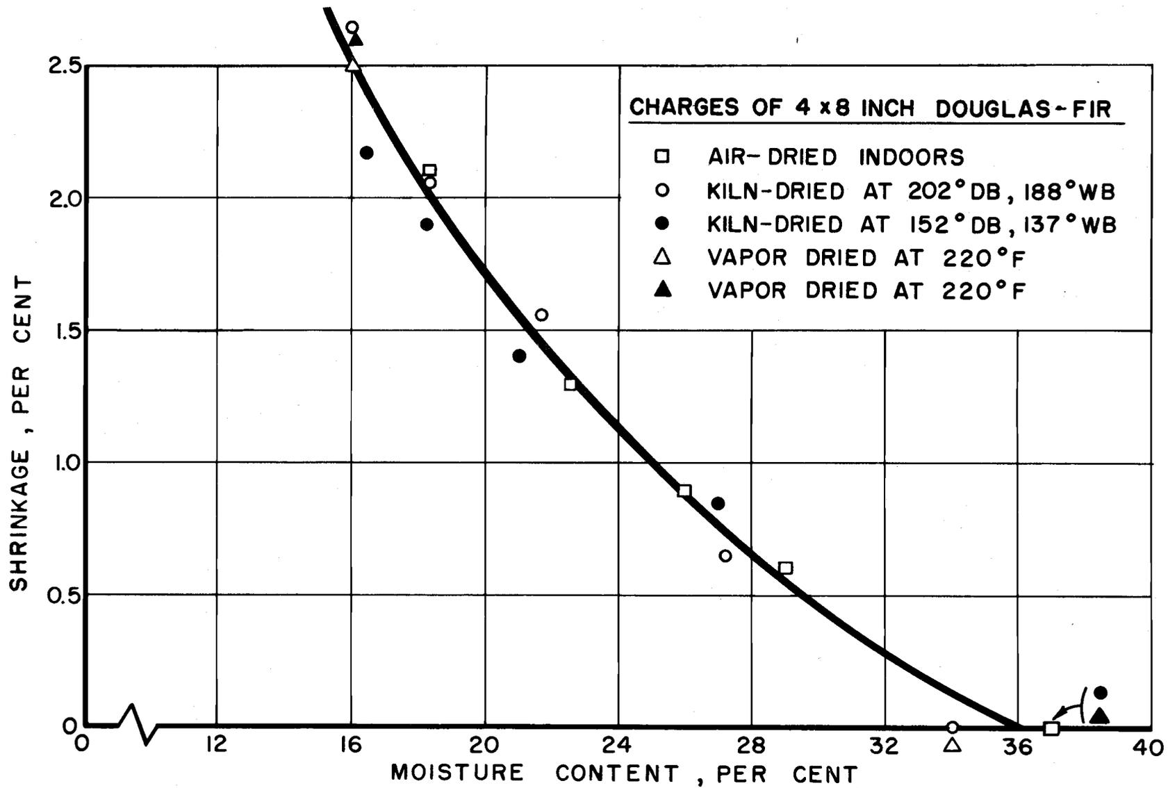
FIGURE 3. SHRINKAGE AND MOISTURE-CONTENT RELATIONSHIPS.
