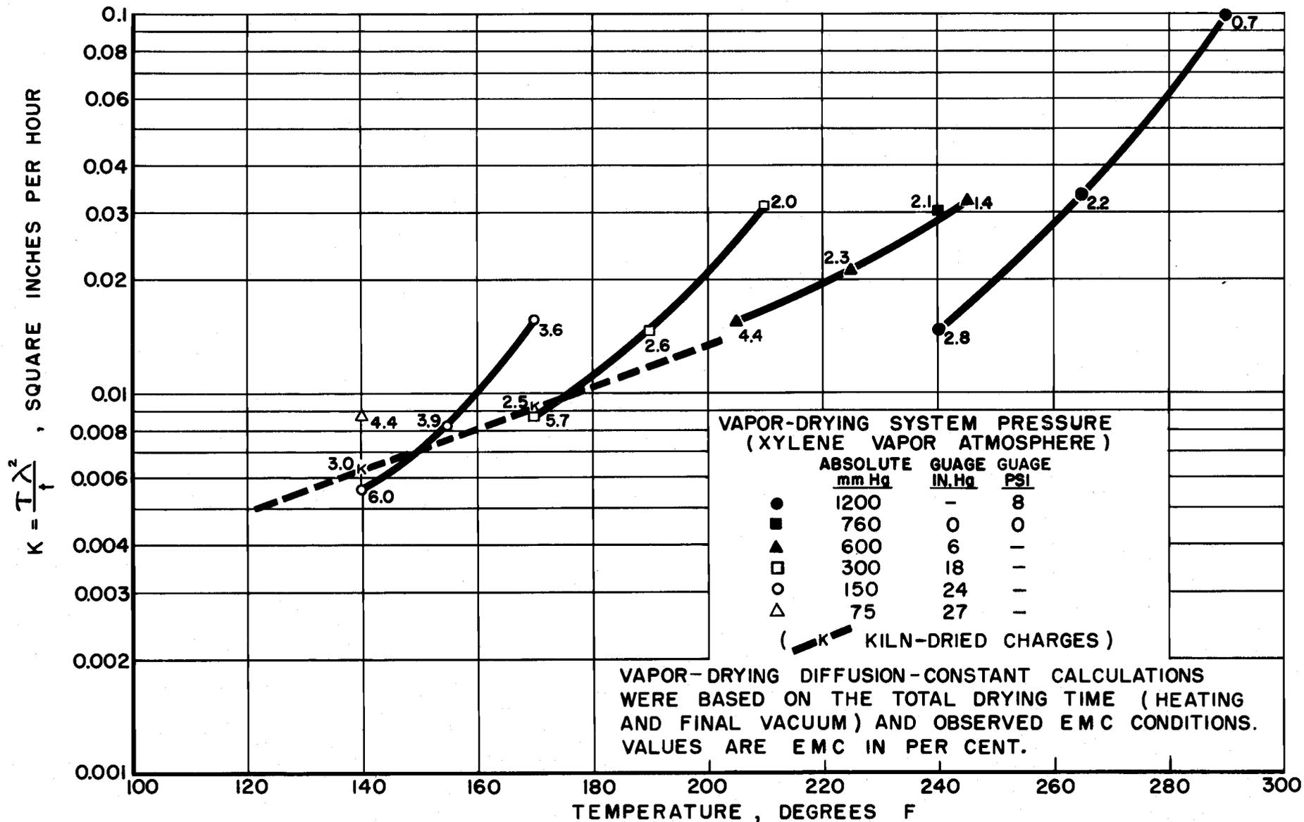
FIGURE 4. TEMPERATURE, PRESSURE AND DRYING-DIFFUSION-CONSTANT RELATIONSHIPS FOR 2-INCH WESTERN HEMLOCK LUMBER.
