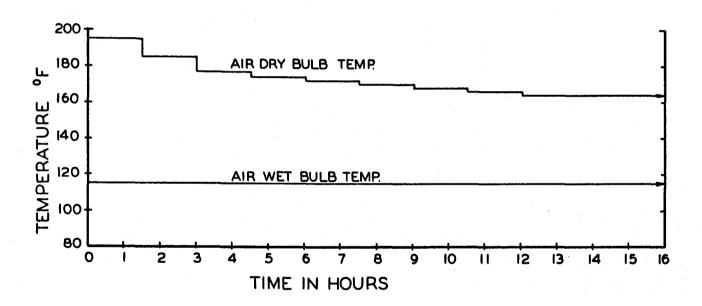
Figure 2. Schedule of Dry Bulb and Wet Bulb Temperatures
