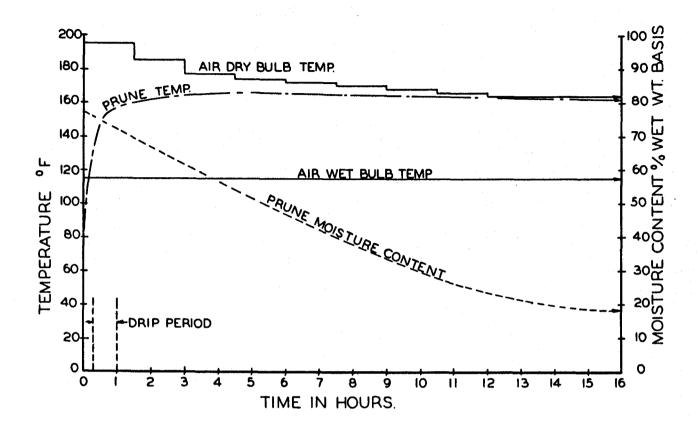
Figure 3. Prune Temperature and Prune Moisture Curves
