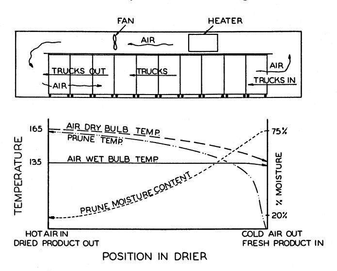
Figure 1. Typical Curves in a Counterflow Dehydration Tunnel for Prunes
